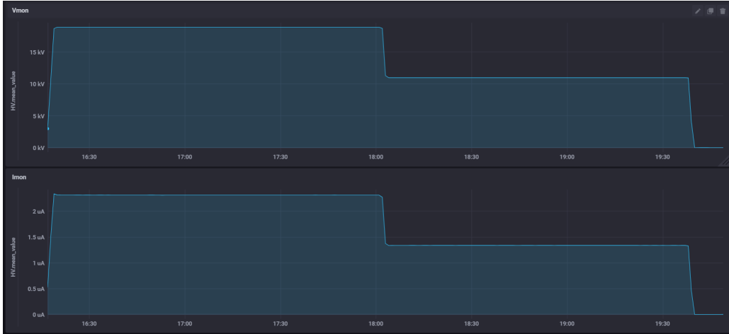
Fig. 4. Example of the voltage (top) and current (bottom) from the Matsusada AU HV power supplies during a data taking run, collected by the P-SCS.
