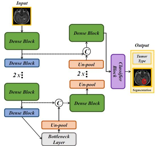
Fig. 1. Illustration of network architecture consisting of dense, bottleneck and classifier blocks shown in the left view. the c in circle symbol represent concat in third dimension. Code available at: [Github Link](#)
