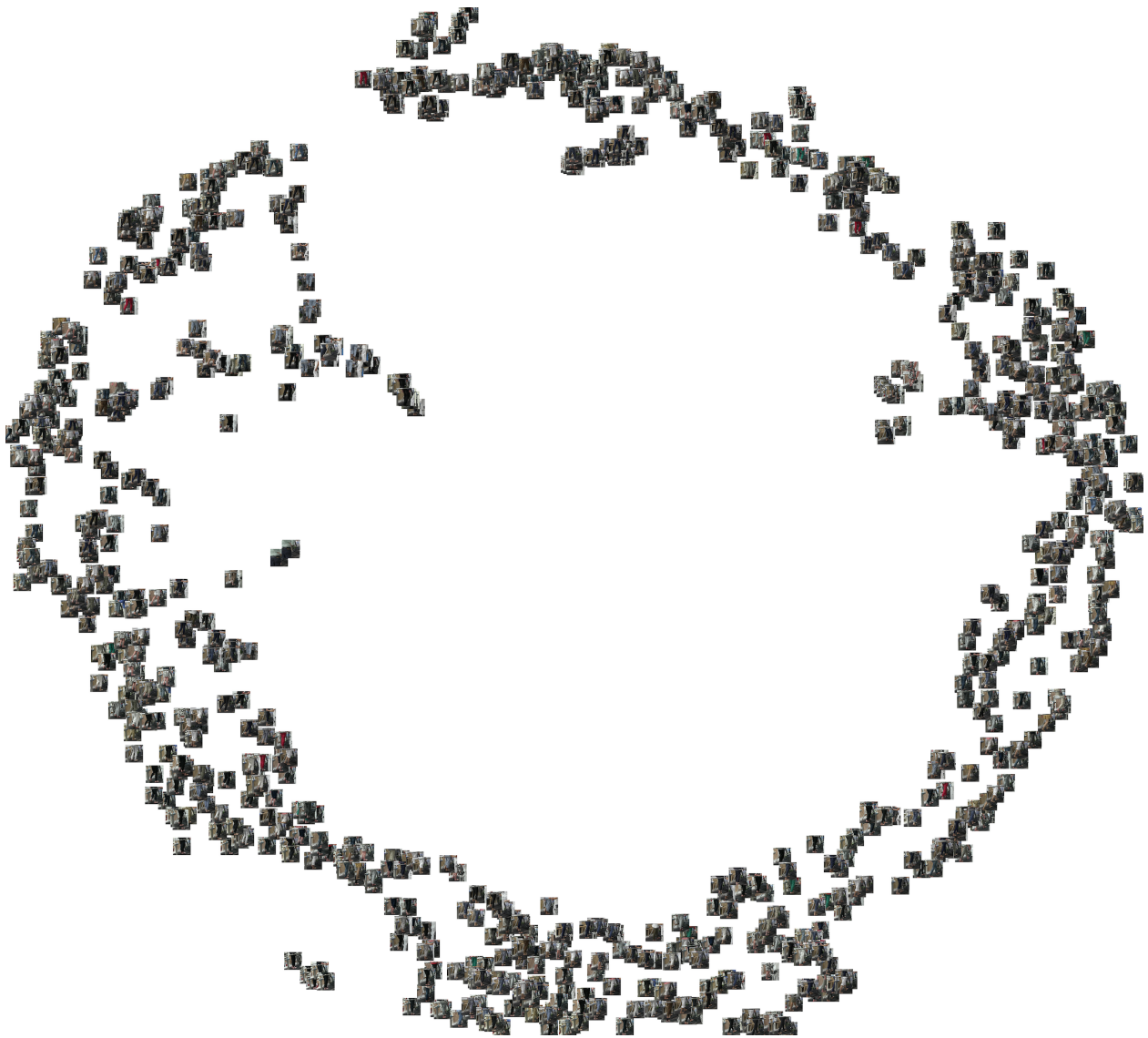
Supplementary Figure 1: Qualitative evaluation of our posture encoding on the human gait dataset. Projection from our posture encoding to a 2D embedding of 1000 randomly chosen postures using tSNE. Similar postures are located close to each other and the walking gait can be reconstructed by following the circle anticlockwise (best viewed by zooming in on the digital version of this figure).
