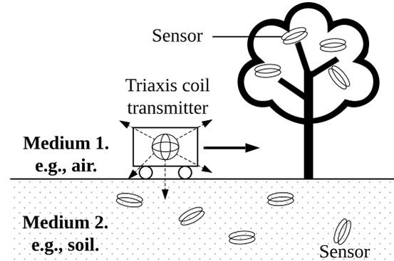
Fig. 1: Illustration of a tri-axis coil in a moving robot being used to charge multiple batteryless sensors with tiny unidirectional coils. The batteryless sensors are used for precision agriculture.
