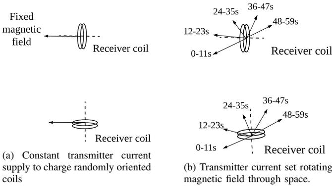
Fig. 3: Illustration comparing performance of constant and rotating magnetic fields for different receiver coil orientations. Fig. 3a shows two instances where maximum voltage is induced when coil axis is aligned with magnetic field (top) and zero voltage induced when coil axis is perpendicular to magnetic field (bottom). Fig. 3b shows how voltage is induced in the receiver coil by the rotating magnetic field at some points during the charging cycle irrespective of coil orientation.
