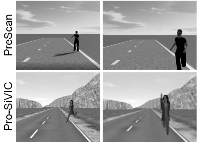
Fig. 3. Crossing pedestrians in PreScan and Pro-SiVIC. Note that we later disabled shadows in PreScan.
