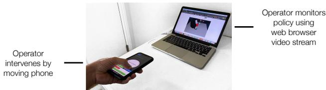
Fig. 2: **System Overview.** We extend the RoboTurk system [26, 28] to enable remote users to monitor policy execution and intervene when they would like to take over control using a web browser and a smartphone. The user monitors policy execution by watching a video stream of the robot in their web browser. They can hold a button on their smartphone to intervene and control the robot by moving their smartphone.
