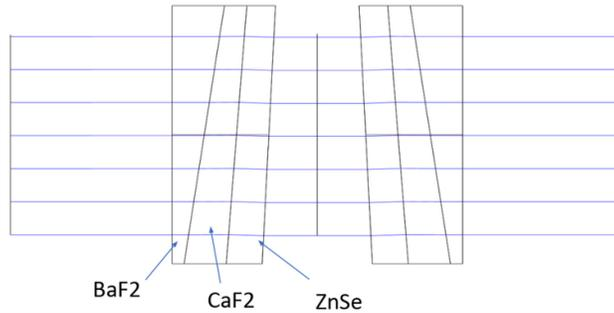
Figure 3. Optical diagram of the ADC design. The three materials that comprise the prisms are labeled.
