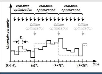
Figure 1: Offline optimal power flow (gray) and online optimal power flow (black).
