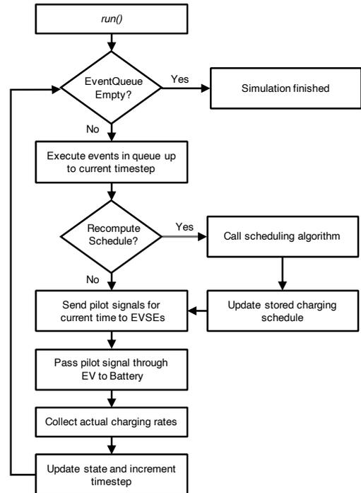
Fig. 3. Flow chart describing the simulator's `run()` function. Each timestep consists of a single iteration of this loop. The simulation ends when the last event from the `EventQueue` is executed at which time the user can analyze the results of the simulation.
