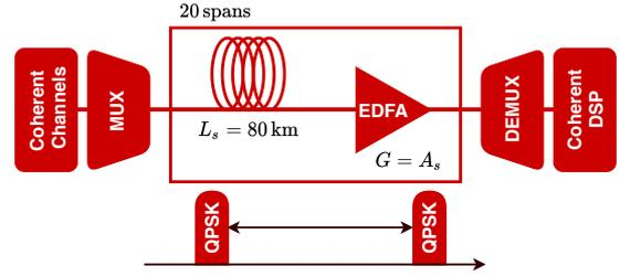
Fig. 1: A sketch of the simulation set-up.
