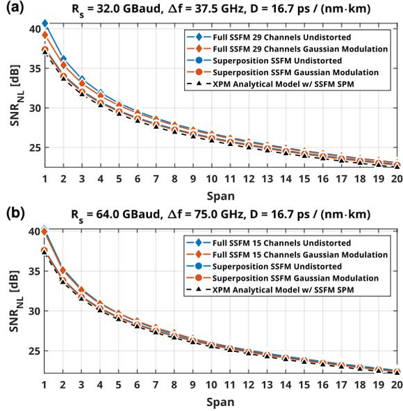
**Fig. 2:** The  $SNR_{NL}$  accumulations for: (a) a widespread use case, and (b) a realistic high symbol rate transmission scenario. A full-spectrum simulation is compared to a superposition of all constituent pump-and-probe simulations, for both predistortion cases.
