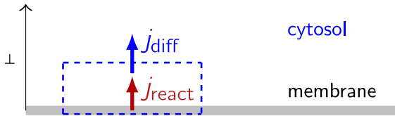
Figure 5. Illustration of reactive boundary conditions. For a given protein state, the net reactive flux from the membrane into the cytosol, j_{\text{react}} , has to equal the cytosolic diffusive flux of that protein state right at the membrane, j_{\text{diff}} . This guarantees local mass conservation: an equal number of proteins flow into and out of the infinitesimal volume indicated by the blue dashed box. The arrow signified with \perp indicates the inward normal on the membrane.
