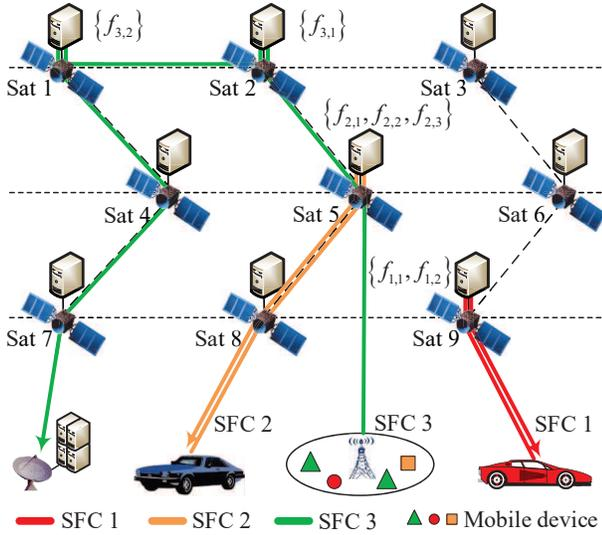
Fig. 3. Example of placing VNFs for three IoT users.
