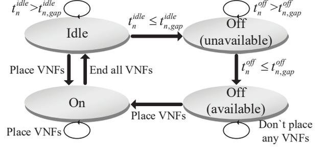
Fig. 2. State transition diagram of an edge server.
