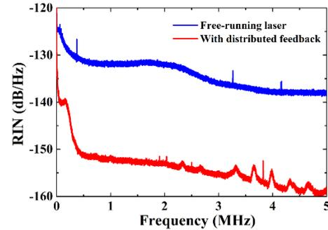
**Fig.7** Comparative curves of the RIN spectrum
