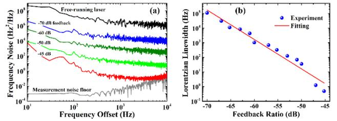
**Fig.5** (a) Evolution curves of the frequency noise PSD under different feedback ratio, (b) Evolution curves of output linewidth with the feedback ratio.
