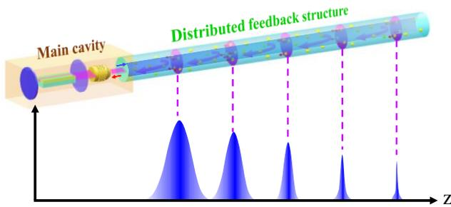
**Fig.1** A novel laser structure assisted by a distributed feedback.
