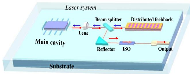
**Fig.3** An on-chip laser system based on distributed feedback external cavity structure
