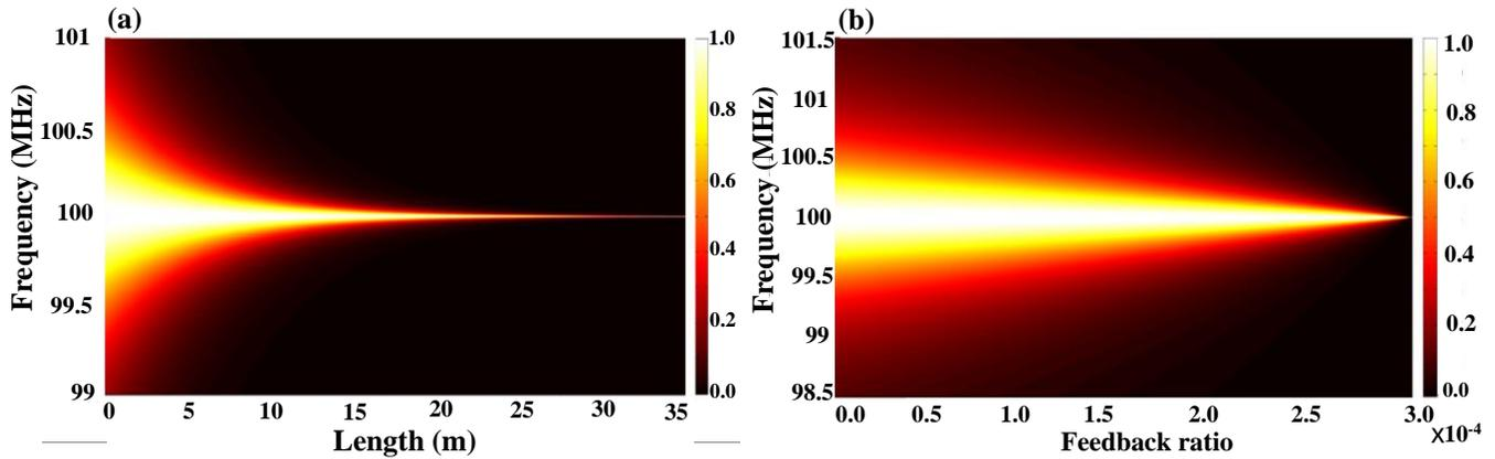
**Fig.2** Simulation results of linewidth evolution. (a) Compression characteristics of laser linewidth caused by the length change of distributed feedback, (b) Compression characteristics of laser linewidth caused by the feedback ratio of distributed feedback
