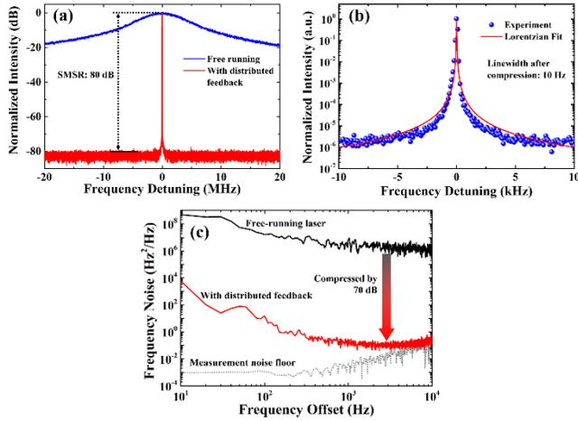
**Fig.4** (a) Comparison curves of the frequency spectrum from beat frequency signal, (b) Lorentz fitting curve of the linewidth with a distributed feedback, (c) Comparison curves of the frequency noise PSD.
