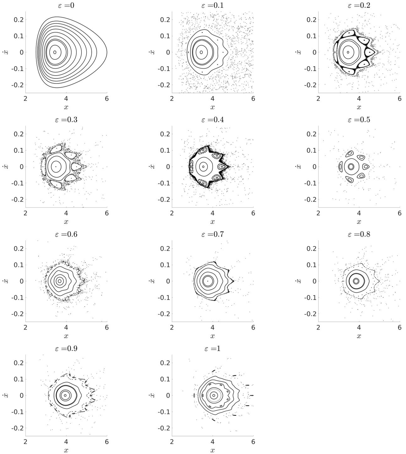
**Figure 7.** The Poincaré map for orbits with  $x_0 = [3.0, 3.5, 3.75, 4.0, 4.25, 4.5, 4.75, 5.0, 5.25, 5.5, 6.0]$  and  $y_0 = 0.0$  as  $\epsilon$  increases from 0 to 1 in steps of 0.1. The system is evolved for 3000 iterations in time-steps of  $\tau = 10$  and the Poincaré map of section for  $y = 0.0, y > 0.0$  is plotted for all 11 initial conditions for the biased-mass system ( $\mu_1 = \mu_2 = 0.001$ ).
