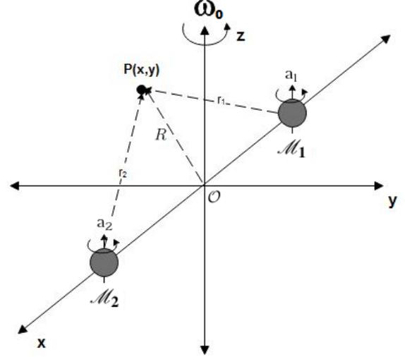
**Figure 1.** The configuration of the two primaries,  $\mathcal{M}_1$  and  $\mathcal{M}_2$ , in the centre-of-mass frame which is rotating about the  $z$ -axis with angular frequency  $\omega_0 (= 1)$ . A test particle with infinitesimal mass  $P$  is placed at an arbitrary position in the equatorial plane.
