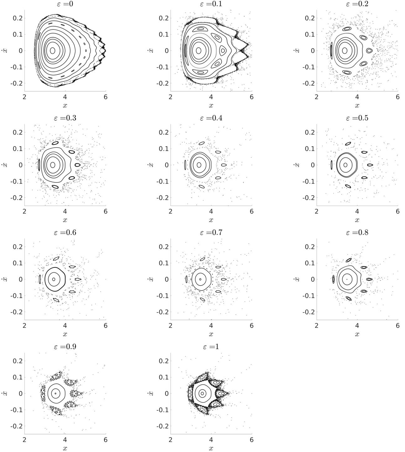
**Figure 8.** The Poincaré map for orbits with  $x_0 = [3.0, 3.5, 3.75, 4.0, 4.25, 4.5, 4.75, 5.0, 5.25, 5.5, 6.0]$  and  $y_0 = [0.0]$  as  $\varepsilon$  increases from 0 to 1 in steps of 0.1. The system is evolved for 3000 iterations in time-steps of  $\tau = 10$  and the Poincaré map of section for  $y=0, \dot{y} < 0$  is plotted for all 11 initial conditions for the Copenhagen system ( $\mu_1 = \mu_2 = 0.5$ )
