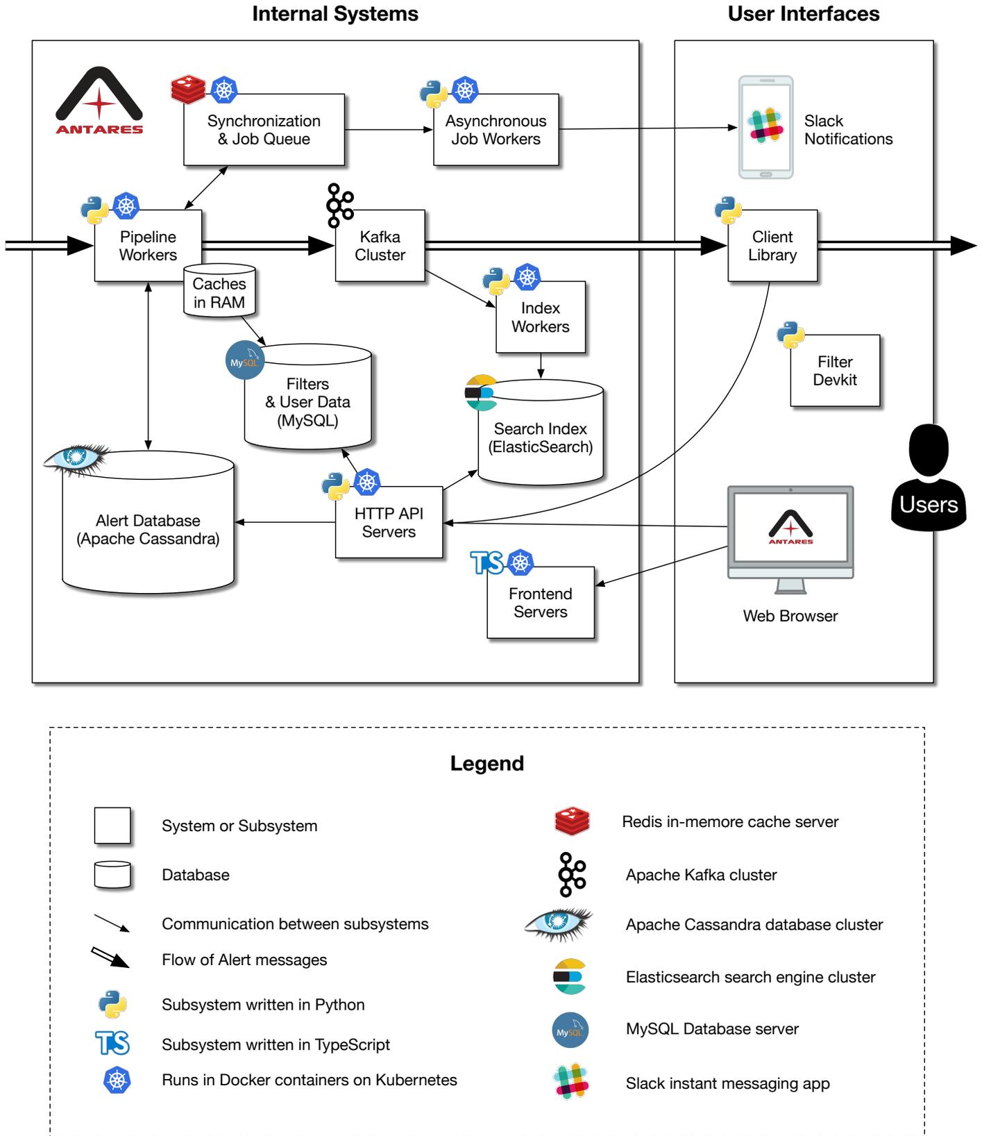
**Figure 3.** Architecture diagram of ANTARES. Input Alerts enter the system on the left (from ZTF, LSST, etc) and output Alerts exit on the right (to downstream systems, TOMs, etc). Many subsystems represent clusters of processes on multiple machines. Subsystems marked with the blue Kubernetes logo run on a shared pool of hardware resources in a Kubernetes cluster. Subsystems not marked with the Kubernetes logo run on dedicated hardware.
