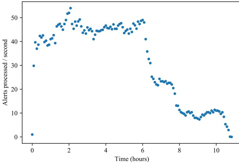
**Figure 5.** Alert throughput over time as ANTARES processes 1.23 million ZTF alerts in approximately 11 hours. The data set was created by merging eight consecutive nights of ZTF data into a single input stream for ANTARES.
