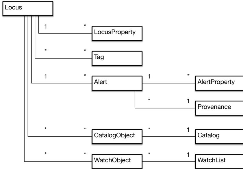
**Figure 1.** ANTARES data model, simplified. Boxes indicate entities. Lines indicate relationships. Asterisks and numbers on lines indicate relationship type: one-to-many (1—\*), many-to-one (\*—1), or many-to-many (\*—\*). Data contained within entities are omitted. The Filter is a software entity, not a data entity, and is also omitted.
