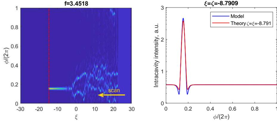
Fig. 5. Left: The field evolution inside the cavity forward wave  $A^+$  with the laser cavity detuning  $\xi$  decrease at  $\beta = 0.037$ ,  $\omega_0 t_s = 0.6\pi/4$ ,  $f = 3.4518$ . The vertical red dash-dotted line is maximum soliton detuning  $\pi^2 f^2/8$ . Right: The azimuthal field profile at the detuning  $\xi \approx -8.8$  together with the theoretical profile of typical secant-square soliton [18] at effective detuning  $\zeta = -8.8$ .
