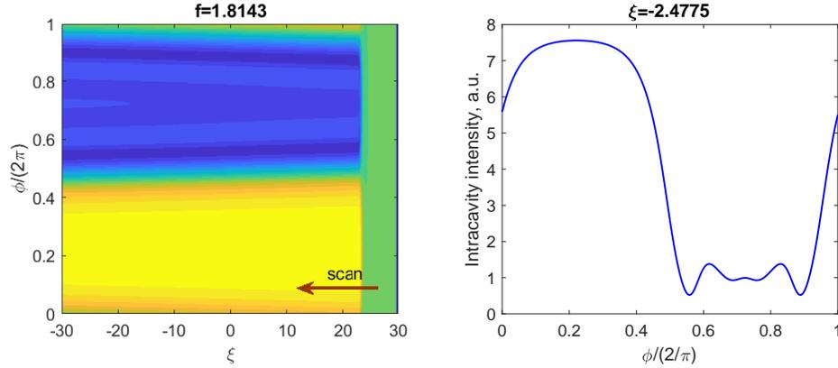
Fig. 8. Left: The forward wave  $A^+$  field evolution inside the cavity with the laser cavity detuning  $\xi$  decrease at  $\beta = 0.1$ ,  $\omega_0 t_s = 3\pi/4$ ,  $f = 1.8143$ . Right: The azimuthal field profile at detuning  $\xi = -2.4775$  (effective detuning  $\zeta \approx -2.72$ ).
