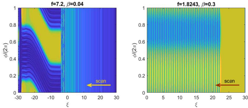
Fig. 11. Left: CW solution instabilities and platicon drift at  $f = 7.2$  and  $\beta = 0.04$ . Right: Breather-like platicon at  $f = 1.82$  and  $\beta = 0.3$ . The locking phase is  $\omega_0 t_s = 3\pi/4$ .
