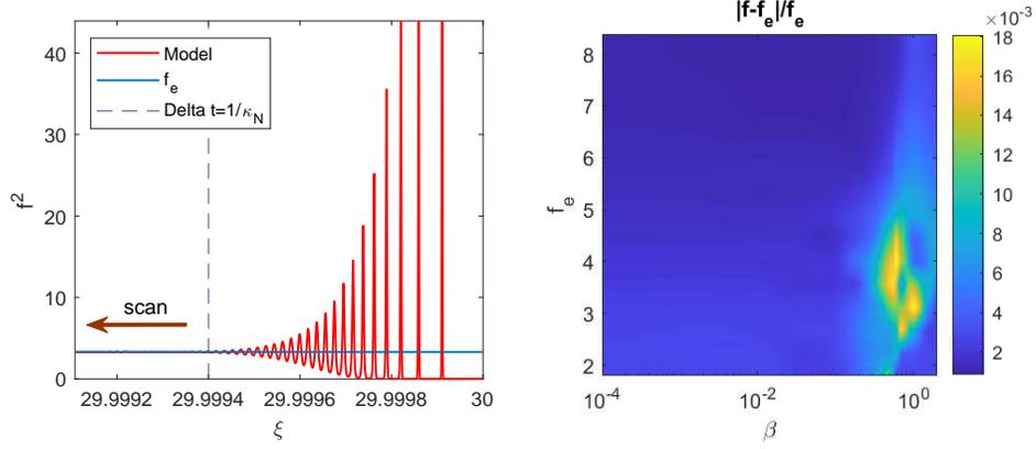
Fig. 1. Left: The start of the laser generation. The actual pump amplitude  $f = f_e a_l$  is shown by the red curve, the blue horizontal line shows  $f_e$  and the vertical dashed line – the detuning after the time, referred to the charge relaxation  $1/\kappa_N$ . Right: average relative deviation of the actual pump amplitude  $f$  from  $f_e$ .
