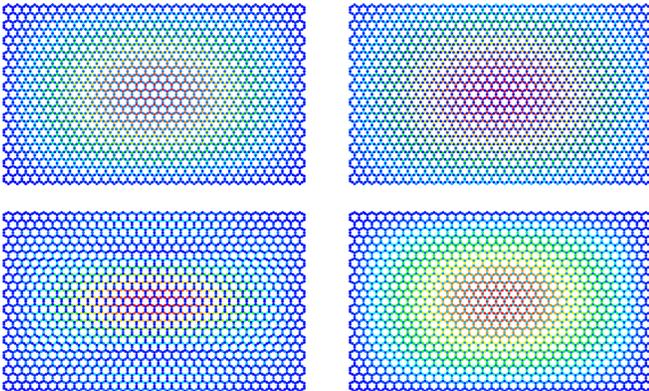
FIG. 9. Eigenmodes with eigenfrequencies of the honome TBM matrix emulating the Dirac microwave billiard at the lower and upper edge of the bands framing the lower DP FB (upper panels), the lower edge of the FB (left lower panel) and upper edge of the bands framing the upper DP (right lower panel). Below the FB the eigenmodes are maximal on honeycomb-sublattice sites. In the other examples they are localized on kagome-sublattice sites. The color code is the same as in Fig. 3.
