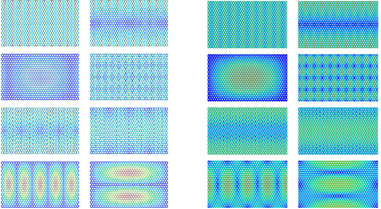
FIG. 12. Eigenmodes with eigenfrequencies of the homone TBM matrix (left part) emulating the microwave Dirac billiard and electric-field intensity distributions (right part) in the microwave Dirac billiard corresponding to resonance frequencies in the bands framing the upper DP. Examples are shown for the regions close to the lower band edge (1st rows), the lower van Hove singularity (2nd rows), the DP (3rd rows) and the upper band edge (4th rows). The color code is the same as in Fig. 3.
