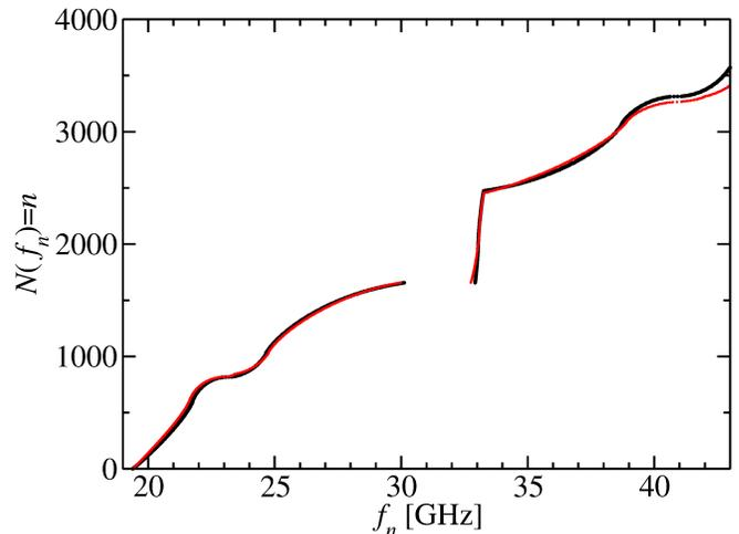
FIG. 10. Integrated DOS of the microwave Dirac billiard (black) and the honome TBM matrix (red). The plateaus correspond to the regions of low spectral density around the DPs, the steep ascend to the region of the FB and the kinks are due to the van Hove singularities.
