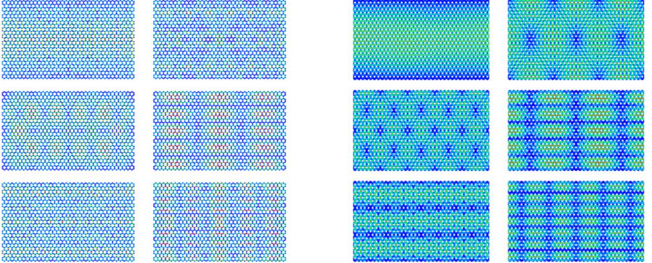
FIG. 13. Eigenmodes with eigenfrequencies of the homone TBM matrix (left part) emulating the microwave Dirac billiard and electric-field intensity distributions (right part) in the microwave Dirac billiard corresponding to resonance frequencies of the microwave Dirac billiard in the FB. The color code is the same as in Fig. 3.
