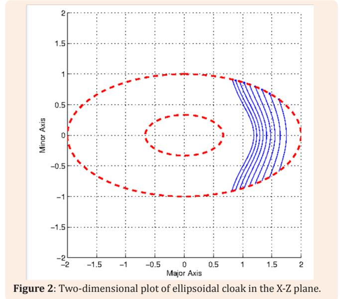
Figure 2: Two-dimensional plot of ellipsoidal cloak in the X-Z plane.
