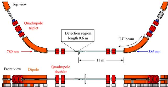
FIG. 2. Top-view and front view of the straight section of the ESR where the laser and the ion beam are superimposed. The lasers are directed through the viewports at the  $60^\circ$ -dipole magnets to co- and counterpropagate with the ion beam.
