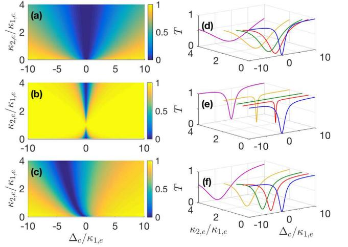
FIG. 3. Pseudo-color maps of transmission rate  $T$  versus detuning  $\Delta_c$  and external decay rate  $\kappa_{2,e}$  with (a)  $\phi = 0$ , (b)  $\phi = \pi$ , (c)  $\phi = \pi/2$ . Profiles of  $T$  versus  $\Delta_c$  with different values of  $\kappa_{2,e}$  and (d)  $\phi = 0$ , (e)  $\phi = \pi$ , (f)  $\phi = \pi/2$ . The other parameter is  $\kappa_{c,i}/\kappa_{1,e} = 0.1$ .
