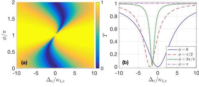
FIG. 2. (a) Pseudo-color map of transmission rate  $T$  versus detuning  $\Delta_c$  and phase  $\phi$ . (b) Profiles of  $T$  versus  $\Delta_c$  with different values of  $\phi$ . The other parameters are  $\kappa_{c,i}/\kappa_{1,e} = 0.1$  and  $\kappa_{2,e}/\kappa_{1,e} = 1$ .
