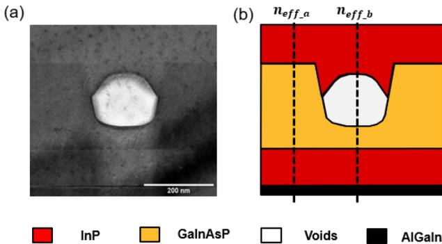
Figure 2: a) A TEM image, and b) a schematic of one re-grown circular etched feature in the photonic crystal pattern. The etched GaInAsP can be seen, as well as the regrown InP that fills this etched feature, and a central air-void. The dotted lines in b) denote the cross section from which the effective refractive indices used in further simulations are taken.
