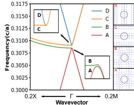
Figure 3: a) The band structure around  $\Gamma$ -point band edges of a square lattice, circular unit cell photonic crystal, with insets showing degeneracy of the bands and the in plane electric field of each band shown adjacent, the black circles represent the edge of the refractive index contrast in the photonic crystal, and the arrow size represents the intensity of the electric field at each point
