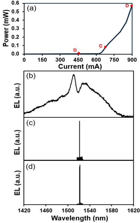
**Figure 4:** a) The current-power characteristics of an InP-based PCSEL, measured under pulsed conditions (10% duty cycle, 10  $\mu$ s pulse width). b), c) and d) show the emission spectra of the device when driven at 450 mA, 700 mA, and 900 mA respectively.
