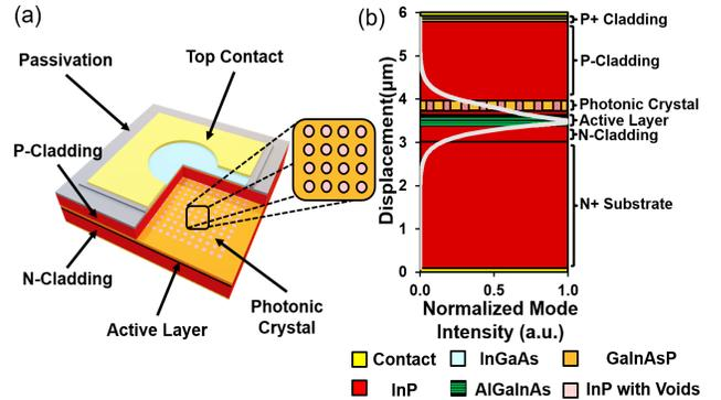
**Figure 1** a) A schematic of the device, with cut-out area showing the photonic crystal pattern and active layer. b) A schematic of the corresponding mode distribution inside the device structure. The epitaxial structure is shown, with the various materials in the key below.
