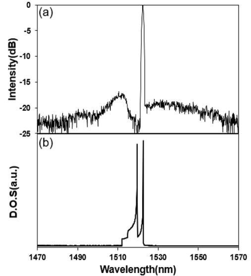
**Figure 5:** a) The emission spectrum of a typical device, plotted from 1470 nm to 1570 nm. b) The corresponding simulated optical density of states.
