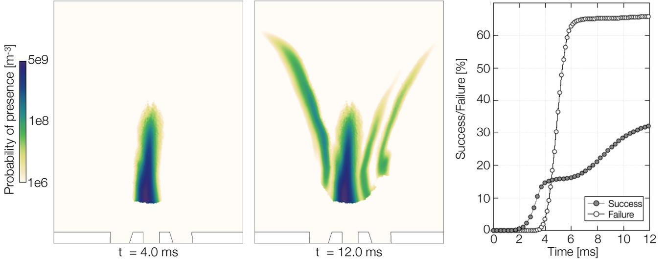
Figure 13:  $P$  Case. Probability density of successful ignition,  $p_s(\mathbf{x}, t)$  in a central cut-plane at two instants for sparking at  $(r/D_{ext} = 0.0, z/D_{ext} = 1.4)$ , and temporal evolution of  $P_s(t) = \int_V p_s(\mathbf{x}, t) dV$  and  $P_f(t) = \int_V p_f(\mathbf{x}, t) dV$ .
