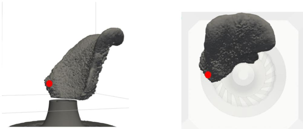
Figure 16: *SP* case. Prediction of MIST for sparking at  $(r/D_{ext} = 1.5, z/D_{ext} = 0.5)$  (red dot) : final ( $t = 12$  ms) iso-surface of all positions where  $r_s$  was reached. Left: side view; Right: top view.
