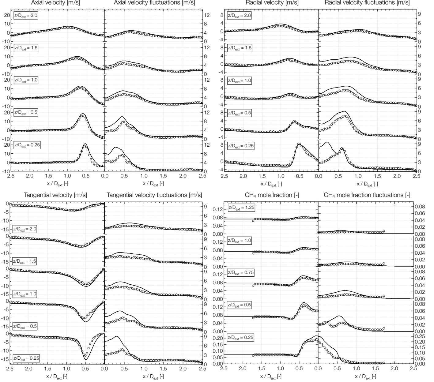
Figure A.18: Comparison of time-averaged velocity and fuel mole fraction mean and fluctuating profiles from non-reacting LES against experimental data at 5 axial locations.
