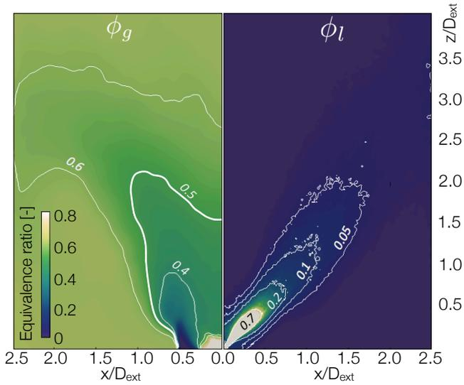
Figure 4: *SP* case. Maps of the cold flow gaseous equivalence ratio  $\phi_g$  (left) and liquid equivalence ratio  $\phi_l$  (right). The highlighted  $\phi_g = 0.5$  corresponds to the lean flammability limit of *n*-heptane which also marks the transition between weakly evaporation-controlled flames ( $\phi_g > 0.5$ ) and evaporation-controlled flames (Section 3.2.1).
