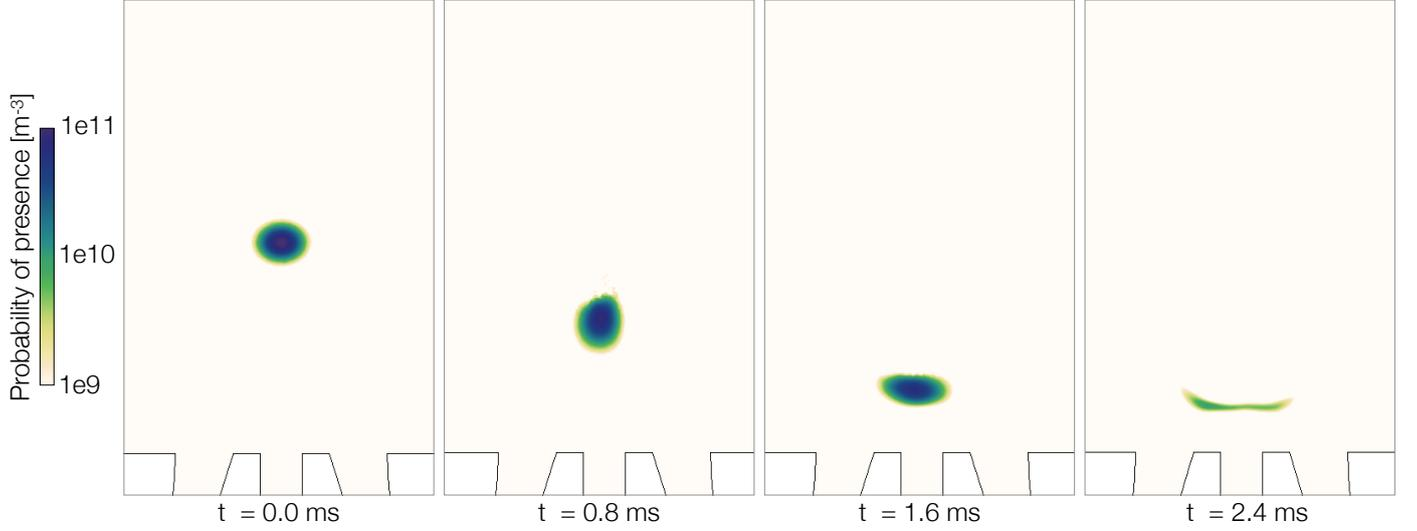
Figure 12:  $P$  case. Probability density of presence  $p(\mathbf{x}, t)$  of all size kernels in a central cut-plane at four instants for sparking at  $(r/D_{ext} = 0.0, z/D_{ext} = 1.0)$ .
