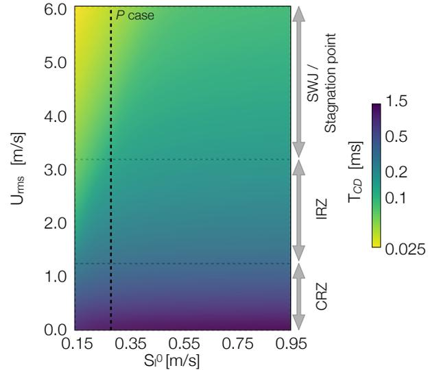
Figure 5: Kernel cooling time  $t_{CD}$  map as function of  $S_L^0$  and  $u'$  for an initial methane/air kernel with a spark energy of 30 mJ. The vertical dashed line corresponds to the  $P$  case laminar flame speed. The vertical arrows indicate typical range of  $u'$  in distinct areas of the swirled flow (see Fig. 2).
