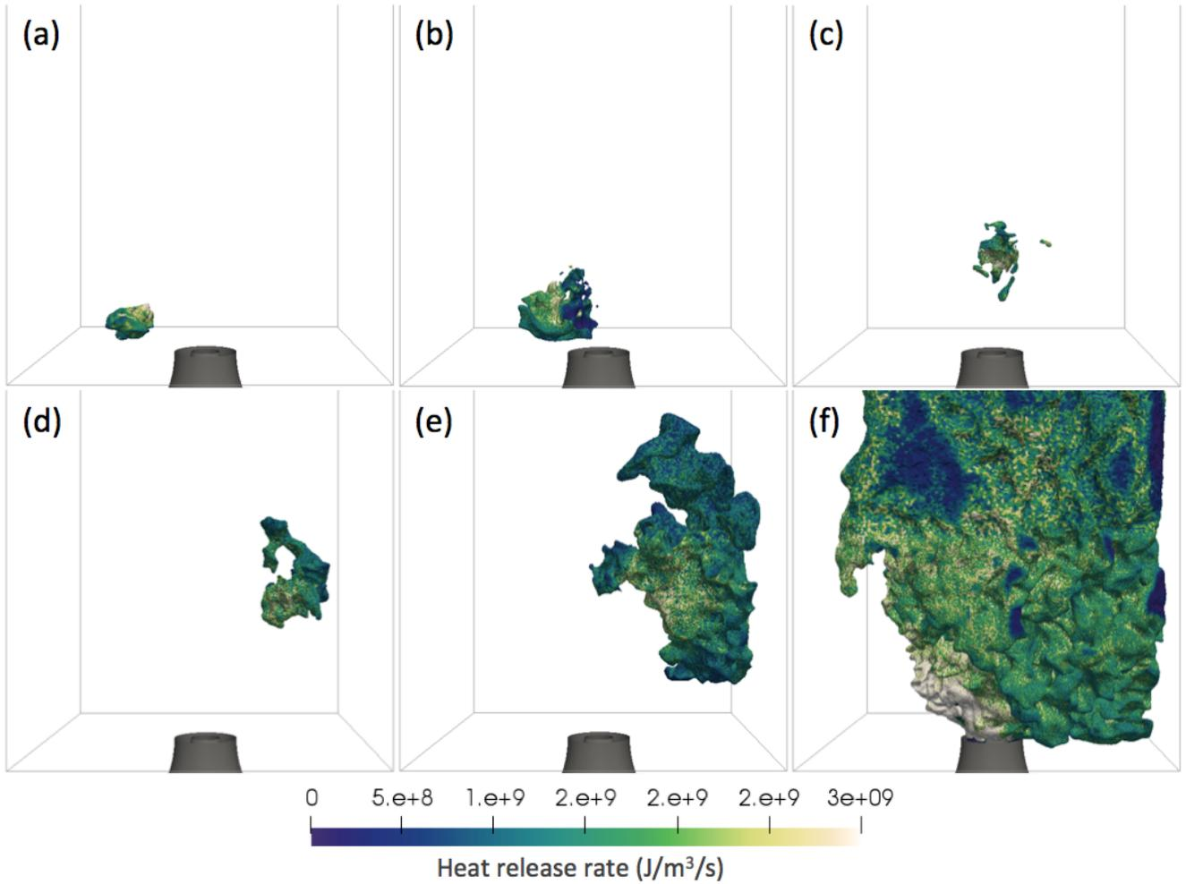
Figure 15: *SP* case. Snapshots of LES for sparking at  $(r/D_{ext} = 1.5, z/D_{ext} = 0.5)$ . Flame front visualization ( $iso-T = 1500$  K) colored by heat release rate. Time after spark: (a) 1.7 ms, (b) 3.7 ms, (c) 7.7 ms, (d) 13 ms, (e) 16 ms, (f) 20 ms.
