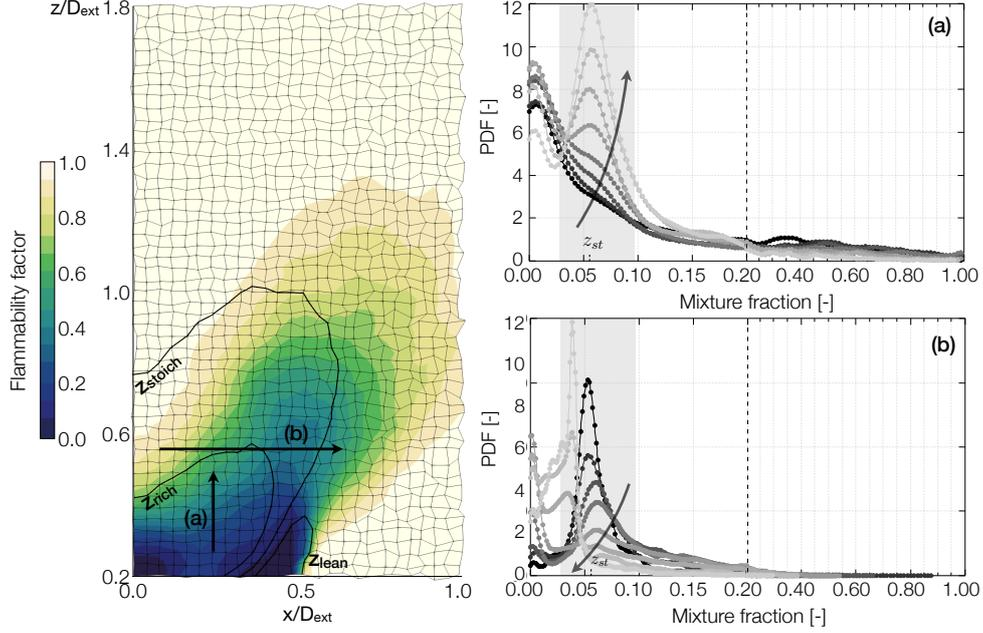
Figure 3: *NP* case. Mean flammability factor field in a central  $x$ -normal plane with  $Z$  iso-lines (left) and  $P(Z)$  along arrows (a) (top) and (b) (bottom) in the mixing region (right). The grey area highlights the flammable mixture interval.
