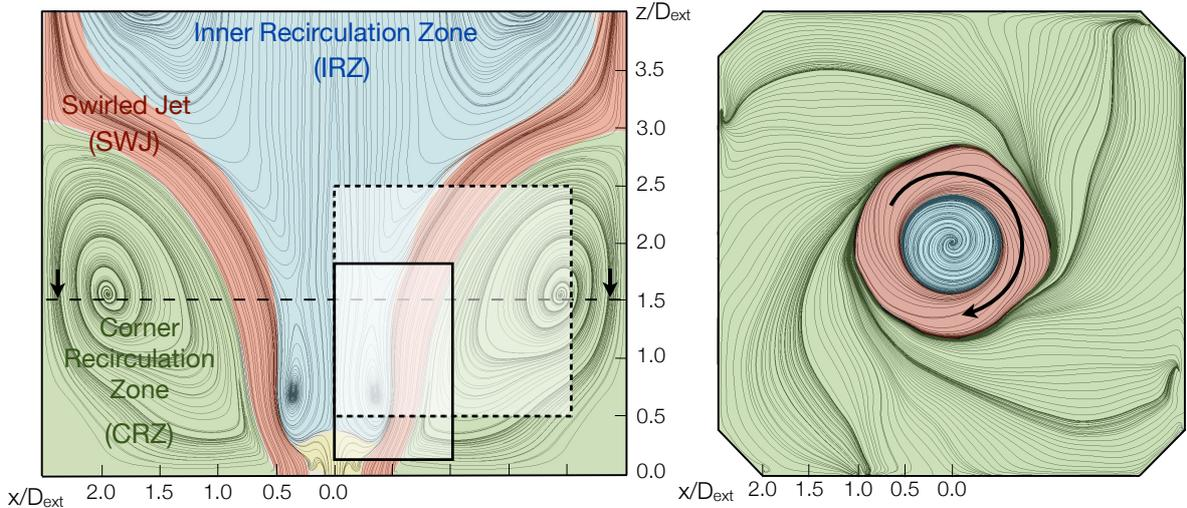
Figure 2: *NP* case, non-reacting flow. Time-averaged pseudo-streamlines in a central *x*-normal plane (left) and *z*-normal plane (right). Swirled Jet (SWJ, red), Inner Recirculation Zone (IRZ, blue) and Corner Recirculation Zone (CRZ, green). Boxes respectively indicate the experimental ignition maps for *P*, *NP* (plain) and *SP* (dashed) cases.
