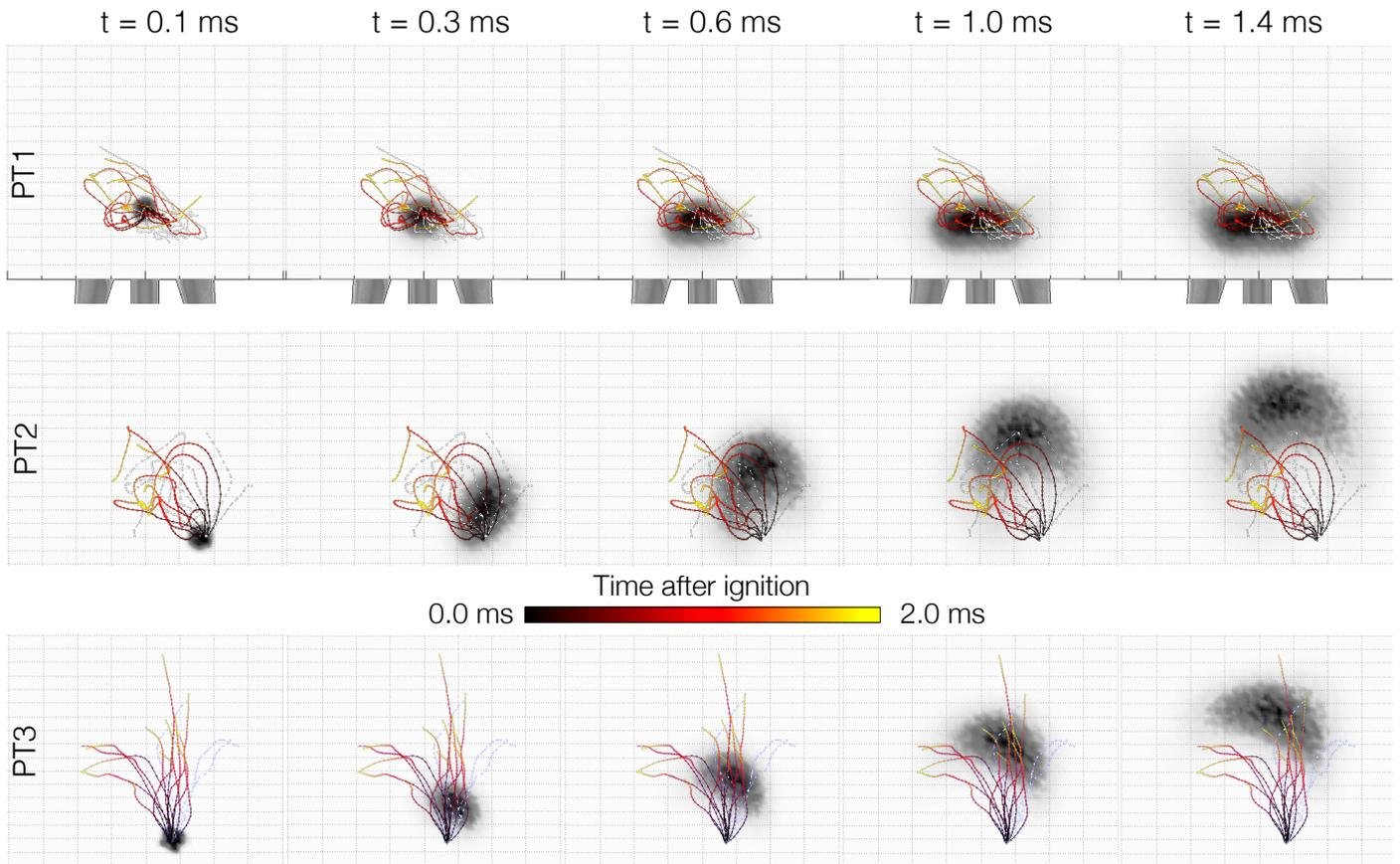
Figure 14: NP case. Two-dimensional projection of  $p(\mathbf{x}, t)$  of all size kernels obtained from MIST (grayscale) with overlaid kernel trajectories obtained from LES (lines) colored by the time after ignition.
