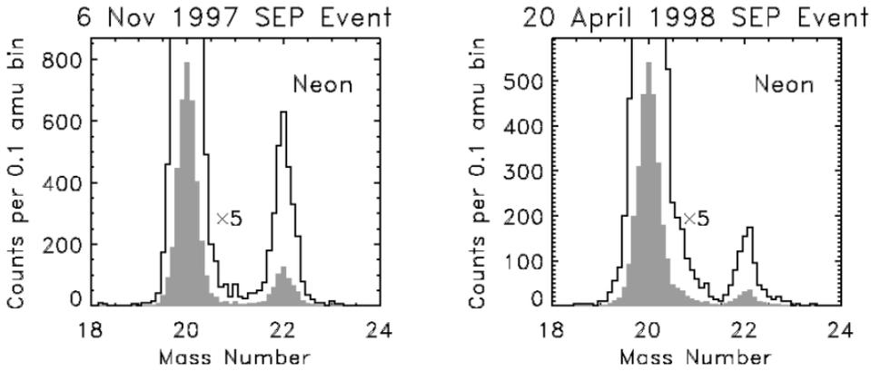
**Fig. 7.5.** Panels show the resolution of Ne isotopes by the SIS telescope in two SEP events. Histograms are also shown enhanced by a factor of 5 to clarify  $^{22}\text{Ne}$  measurement (Leske et al. 2007 © Springer). Isotope measurements show  $A/Q$  enhancements like those in element abundances.
