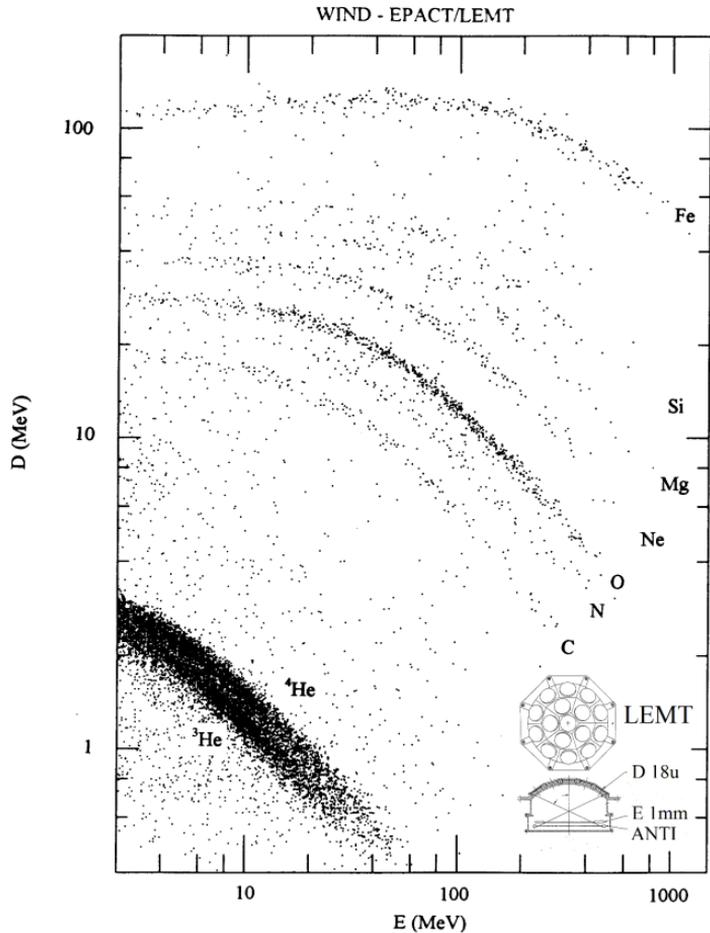
Particles entering LEMT are corrected for angle of entry, mapped in a  $\log D$  vs.  $\log E$  space, like that of Fig. 7.3, and binned onboard according to particle species and energy interval (see Reames, Ng, and Berdichevsky 2001). The right-hand ends of the particle tracks, especially noticeable for C, N, and O, occur just before the ions have enough energy to begin to penetrate into the anticoincidence detector.
