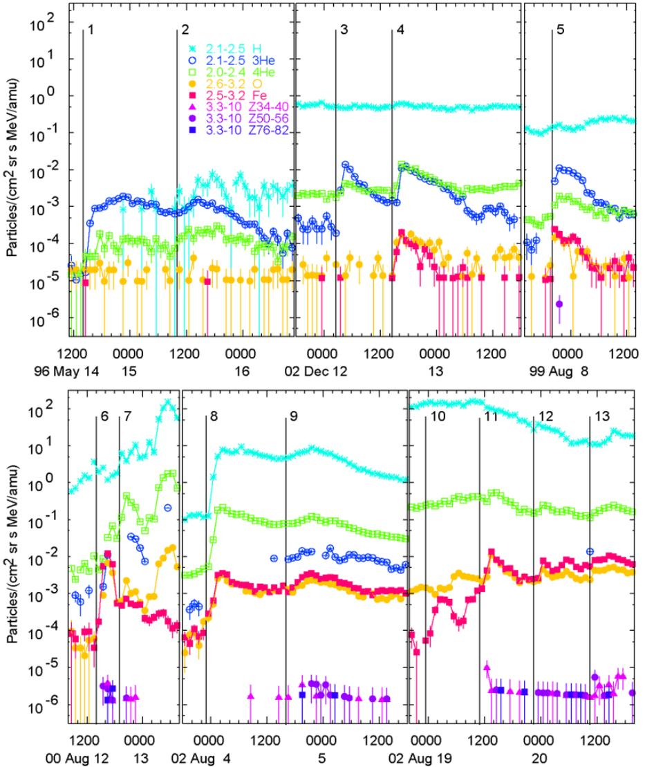
**Fig. 4.2** Intensities of H,  $^3\text{He}$ ,  $^4\text{He}$ , O, Fe, and heavy elements are shown as a function of time during 13 impulsive SEP events (see text, Reames and Ng 2004 © AAS).
