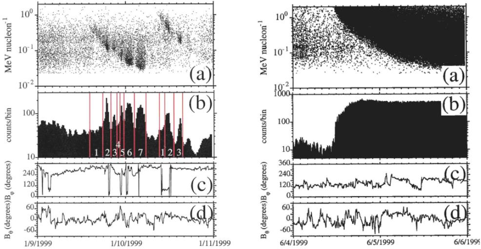
**Fig. 3.8** Panels (a) show the energy vs. the arrival time of individual ions from an impulsive (*left*) and a gradual (*right*) SEP event. Panels (b) show the corresponding ion count rates while (c) and (d) show the magnetic field direction. Particles or gaps occur because some flux tubes connect to the compact source of impulsive SEPs and others do not (Mazur et al. 2000, © AAS).
