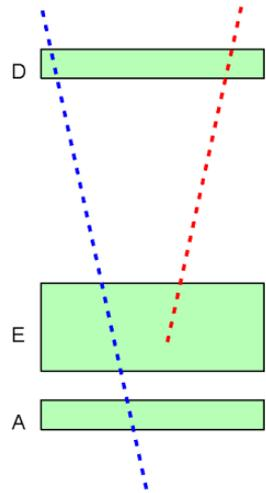
Most of the particle telescopes flown in space are of this general type, although multiple detectors may be used in place of the D and E elements. Early telescopes used plastic scintillator or even gas drift chambers, but most telescopes of the last 25 years are “solid state” Si detectors which have extremely high resolution and *stability*, *i.e. their response does not change at all during decades of operation*. Gas detectors soon suffer from out-gassing, contamination, or leakage.
