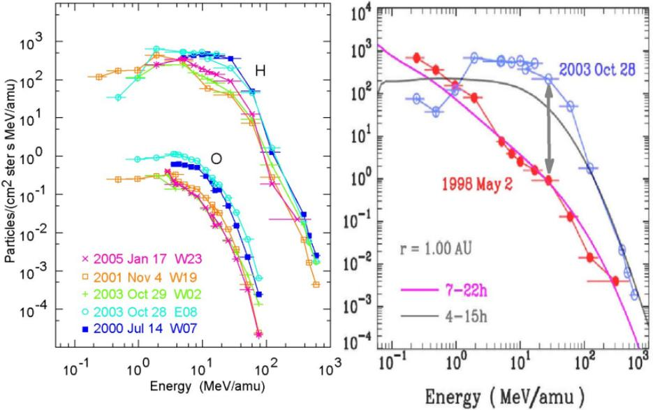
**Fig. 5.5.** The *left panel* shows energy spectra of H and O in five large gradual SEP events (all GLEs) that are flattened at low energies (Reames and Ng 2010 © AAS). The *right panel* shows that the small event of 2 May 1998, with greatly reduced H intensities at 10–100 MeV (*gray arrows*), cannot generate enough waves to suppress lower energies. Model fits to the spectra are shown in *gray and purple curves* (see Ng, Reames, and Tylka 2012).
