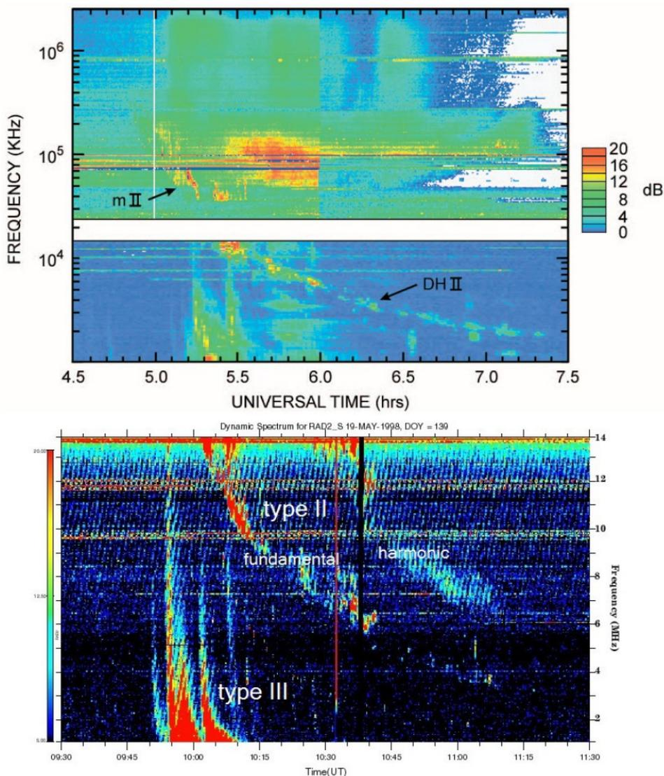
**Fig. 2.1** The *lower* panel shows the dynamic radio spectrum obtained by the *Wind*/WAVES instrument in May 1998 with type II and type III bursts. The *upper panel* shows the type II burst associated with the large SEP event of 26 December 2001 as it propagates from the ground-based metric ( $\geq 25$  MHz) Hiraizo station to the *Wind*/WAVES decametric-hectometric DH ( $\leq 14$  MHz) regime (Cliver, Kahler, and Reames 2004, © AAS).
