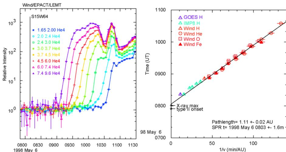
**Fig. 3.1** The *left panel* shows the arrival of  $^4\text{He}$  ions of the indicated  $\text{MeV amu}^{-1}$  intervals at the *Wind* spacecraft near Earth. The *right panel* shows the onset time of these and other intervals vs.  $v^{-1}$ . For the fitted line, the slope is the pathlength and the intercept is the solar particle release (SPR) time at the Sun for this large gradual GLE event (Reames 2009a, © AAS).
