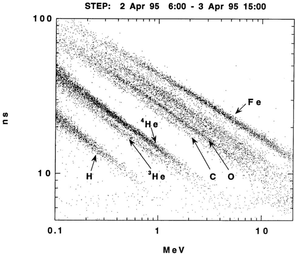
**Fig. 7.7.** The response of the STEP telescope shows the time-of-flight (ns) vs. the total kinetic energy (MeV) for a sample of ions during a small  ${}^3\text{He}$ -rich SEP event (see von Rosenvinge et al. 1995; Reames et al. 1997 © AAS).
