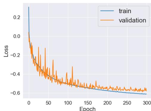
**Fig. 4.** MDN Loss ( $-\log(\mathcal{L})/N$ ) as a function of epoch. The loss obtained during the MDN training and validation are shown by blue and orange lines, respectively.
