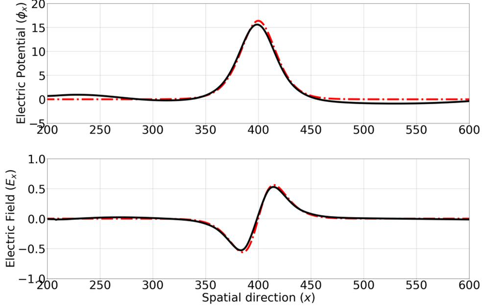
**Figure 3.** The electrostatic potential/E-field profile of EH1 is shown in the top/bottom panel. The initial condition i.e. at  $\tau = 0$  (red dotted curve) is compared with  $\tau = 12.0$  (solid black curve), showing a good agreement and hence confirming the stability of EHs during long-time propagation.
