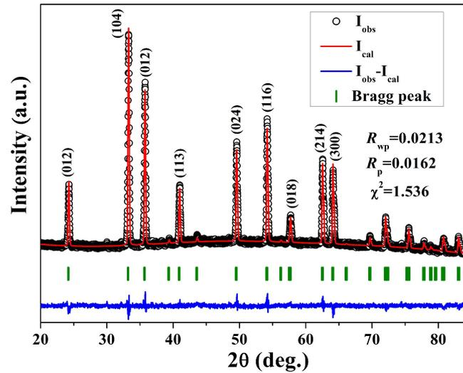
**Fig. 1.** The X-ray pattern was refined using GSAS-EXPGUI program based on the Rietveld method, the Miller indices of the Bragg peaks are also shown. The Rietveld profile fitting parameters are:  $R_{wp} = 0.0213$ ,  $R_p = 0.0162$ ,  $R_e = 0.0139$ ,  $\chi^2 = 1.536$ .
