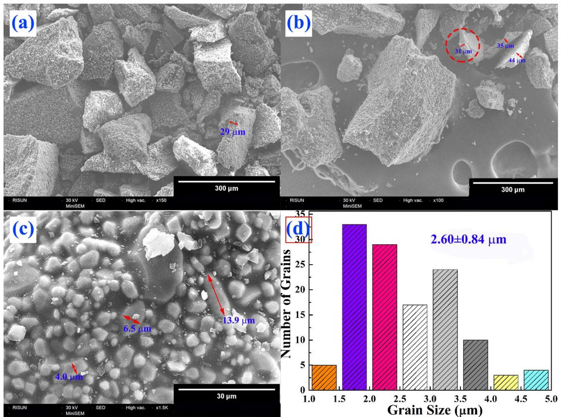
**Fig. 2.** (a) Scanning electron microscopy image of  $\alpha$ - $\text{Fe}_2\text{O}_3$  ceramic sintered at 900 °C and (b) low-magnification and (c) high-magnification images of the ceramic powders and (d) grain size distributions of the particles.
