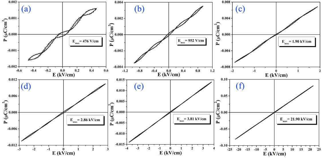
**Fig. 4.** Polarization-electric field hysteresis loops of  $\alpha$ -Fe<sub>2</sub>O<sub>3</sub> at different electric fields and 10 Hz.
