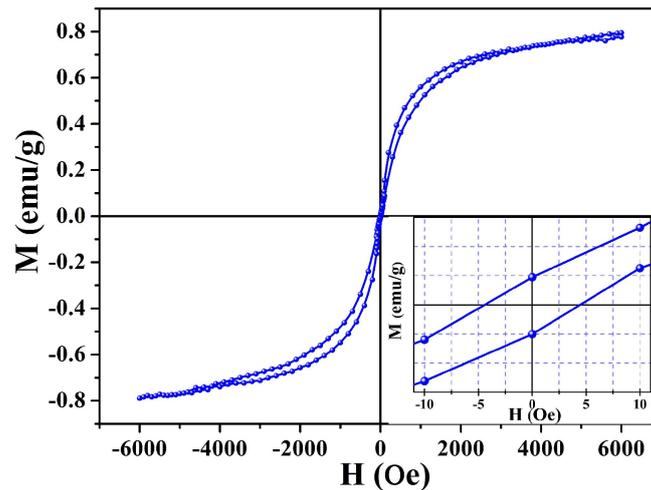
**Fig. 3.** Hysteresis loop of the  $\alpha$ -Fe<sub>2</sub>O<sub>3</sub> powder measured at room temperature.
