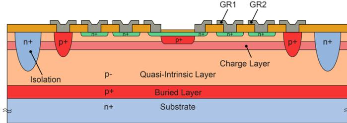
Fig. 2. Cross section of a first-generation red-enhanced SPAD with guard ring structures (GR1 and GR2). Guard rings allow to operate the detector at a voltage larger than the edge breakdown.
