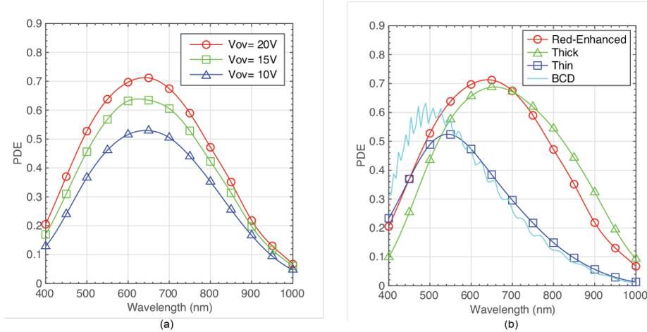
Fig. 9. (a) Photon detection efficiency versus wavelength for the red-enhanced SPAD O25 at three different overvoltages:  $V_{OV}=10V$ ,  $15V$ , and  $20V$ . (b) Photon detection efficiency of different SPADs: a red-enhanced (die O25,  $V_{OV}=20V$ ), a typical custom thin-SPAD ( $V_{OV}=5V$ ), a thick-SPAD from Perkin Elmer Optoelectronics, and a BCD SPAD ( $V_{OV}=5V$ ).
