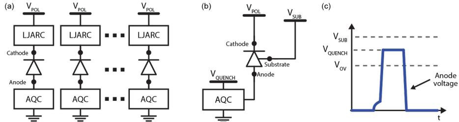
Fig. 3. (a) Typical architecture of a low-jitter SPAD-array, with the Active Quenching Circuit (AQC) and the Low-Jitter Avalanche-Readout Circuit (LJARC) connected at the two terminals of the detector. (b, c) Sketches outlining respectively the different voltages involved in the operation of the SPAD connected to the AQC, and the waveform at the anode.
