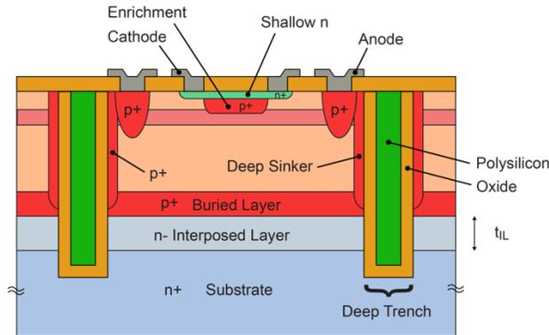
Fig. 4. Cross section of a second-generation red-enhanced SPAD. The  $n^-$  interposed layer increases the anode-substrate breakdown voltage; the deep trenches and the deep sinker provide respectively full electrical insulation between pixels and low series resistance.
