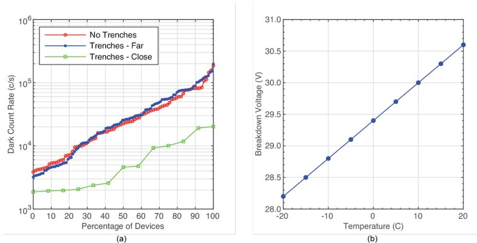
Fig. 7. (a) Distribution of the dark count rate for 50  $\mu\text{m}$  diameter SPADs without trenches (red open circles), with trenches placed far from active area (blue closed circles), and close to the active area (green open squares). All measurements have been performed at an overvoltage  $V_{OV}=15\text{V}$  and a temperature  $T=23^\circ\text{C}$ . (b) Breakdown voltage as a function of the temperature as measured on die O25.
