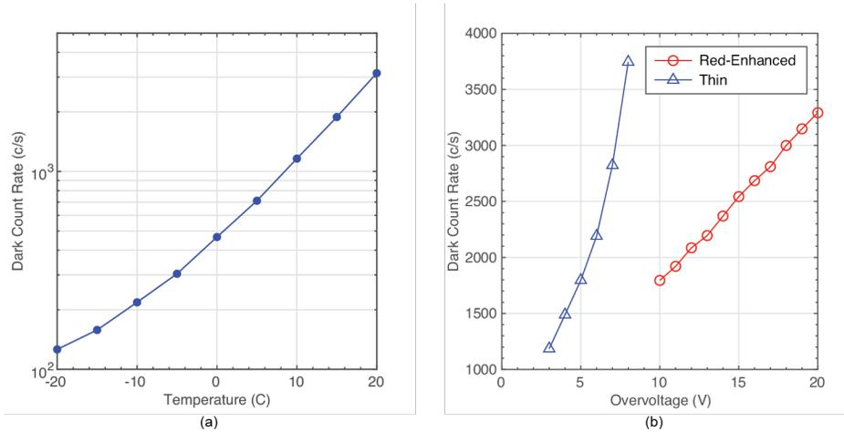
Fig. 8. (a) Dark count rate versus temperature measured on die O25 at  $V_{OV} = 20V$ . (b) Dark count rate versus overvoltage for red-enhanced SPAD O25 and for a typical thin SPAD. Measurements have been performed at temperature  $T = 20^{\circ}C$ .
