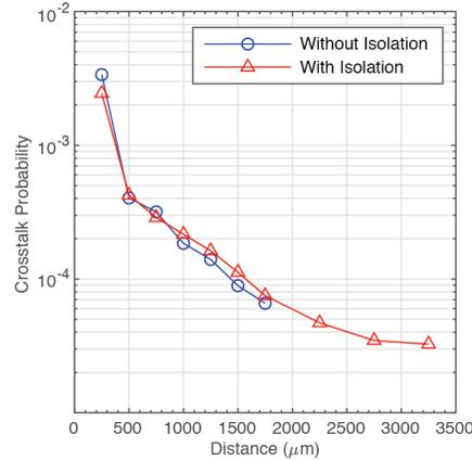
Fig. 11. Optical crosstalk as a function of the distance for RE-SPAD with and without the n+ isolation region ( $V_{ov} = 20\text{V}$ ).
