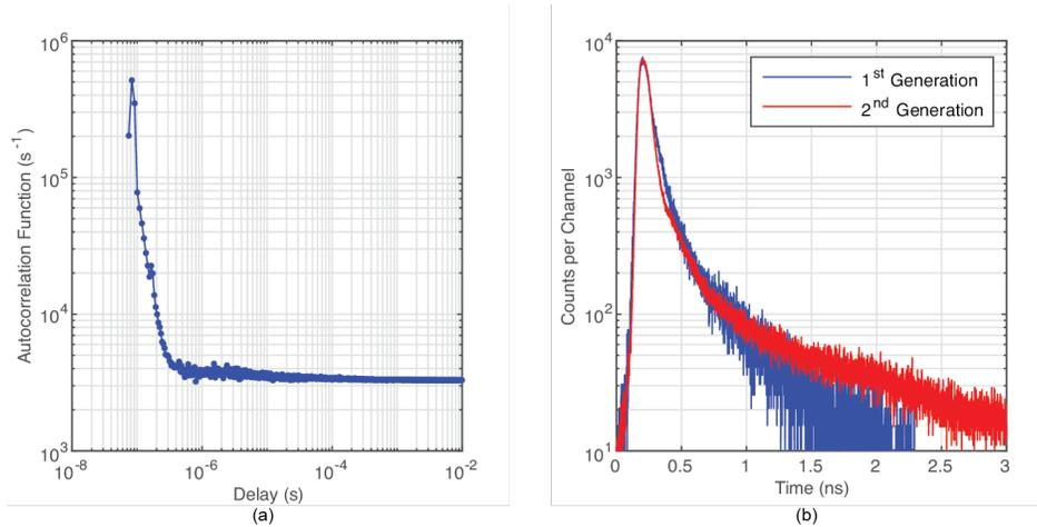
Fig. 10. (a) Autocorrelation function of counts generated in dark condition by red-enhanced SPAD O25 biased at  $V_{ov} = 20V$ . (b) Temporal response of a first-generation (blue curve) and of a second-generation (red-curve) red-enhanced SPAD. The second-generation device attains the same timing jitter of the first-generation one, apart for a longer diffusion tail due to an accidentally thicker buried layer.
