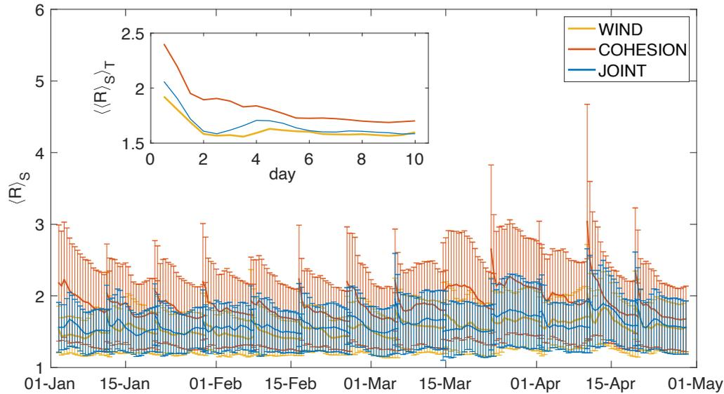
**Figure 9.** Time evolution of the spatial averaged anisotropy of the anisotropic search ellipses. The solid lines indicate the mean and error bars indicate the standard deviation. Inlet: the spatial-temporal domain average of the anisotropy against lead time.
