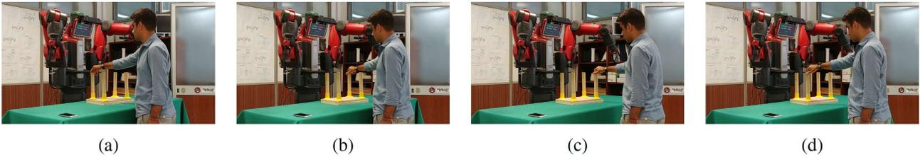
Fig. 13: A sequence of check actions the human operator carries out to verify all connections between the legs and the tabletop.
