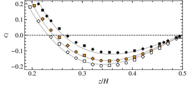
Figure 6. Lift coefficients, Eq. (7), in the channel central portion of the channel at  $Re = 22$  computed using  $a/H = 0.075$ , 0.1, and 0.15 (open, colored, black symbols, respectively). The aspect ratio  $b/a$  is equal to 0.5 (squares), 0.8 (diamonds) and 1 (circles). Dotted curves show calculations from Eq.(3) using Eqs.(A1)-(A3) for  $c_{li}$ .
