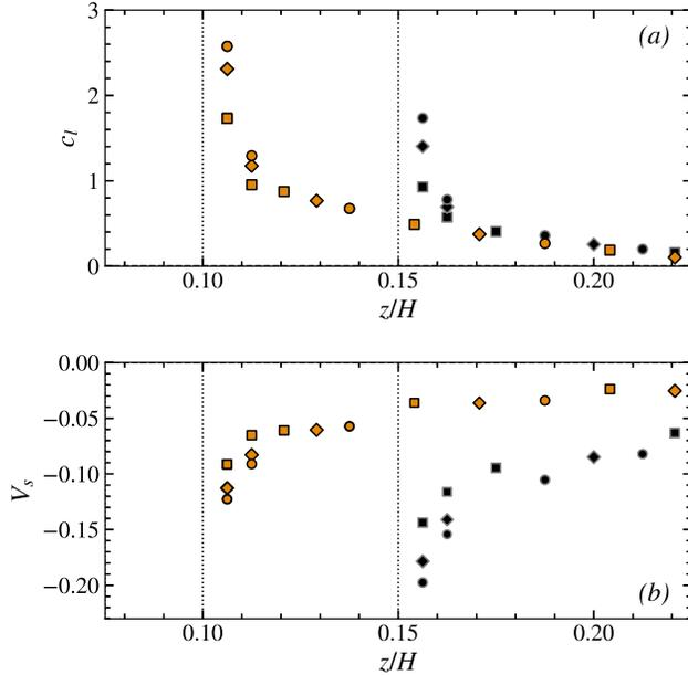
Figure 7. (a) Lift coefficient and (b) particle slip velocity near the wall for spheroids of  $b/a = 0.5$  (squares),  $0.8$  (diamonds) and spheres (circles). Colored and black symbols correspond to  $a/H = 0.1$  and  $0.15$ . Dotted lines indicate a contact with the wall.
