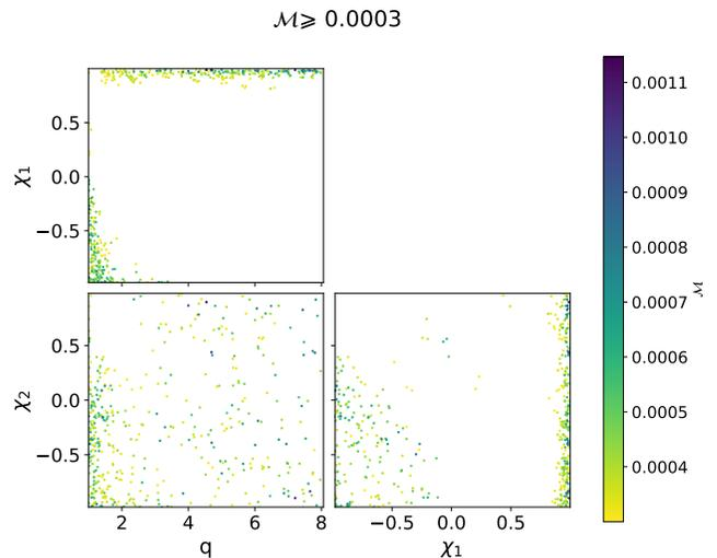
FIG. 3. Mismatches plotted across the  $(q, \chi_1, \chi_2)$  parameter space. Only cases with mismatches larger than the 95th percentile ( $3e-4$ ) are shown. This is the result for  $M_{\text{tot}} = 60M_{\odot}$  but other  $M_{\text{tot}}$  are similar.
