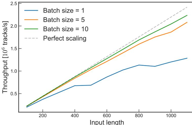
**Figure 11:** Tracks per second processed by the Kálmán filter, as a function of the number of tracks processed in parallel on the tiles (‘input size’). This is given for the cases where multiple ‘batches’ of this size are copied to the tiles before execution. The theoretical maximum throughput evolution as a function of input size is also indicated.
