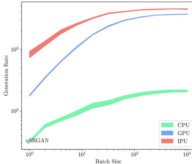
**Figure 4:** Benchmarking the qSRGAN algorithm on CPU, GPU, and IPU processors. The inference throughput for each processor is shown as a function of batch size (left), and the relative ratios shown for the design batch size of one image (right).
