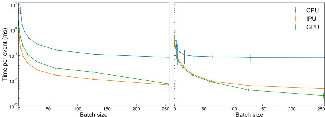
**Figure 6:** Recurrent (left) and convolutional (right) neural network execution time per event as a function of the batch size.
