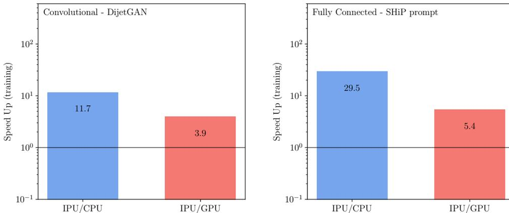
**Figure 5:** Comparison of the time to train the IPU relative to the CPU or GPU of Table 1.
