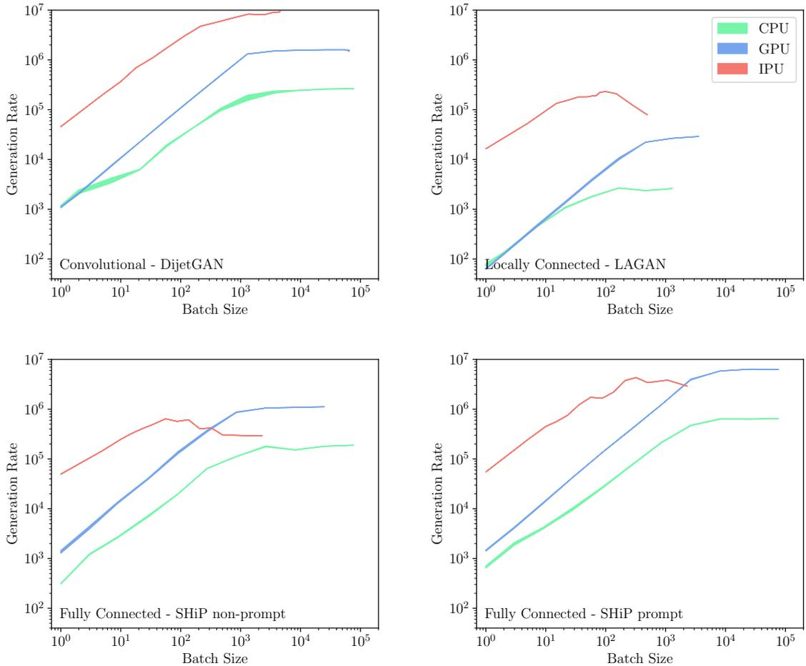
**Figure 2:** Benchmarking results of the event-generation rate as a function of the batch size of the network. Results are presented for IPU, GPU and CPU hardware options outlined in Table 1.
