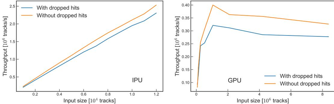
**Figure 12:** Comparison of the throughput with and without conditional execution to ignore mis-associated hits, for a Poplar implementation on the IPU (left), and for a TensorFlow implementation on the GPU (right). The difference in the x-axis scale between the two plots is due to the different memory capacity of the IPU compared to the GPU.
