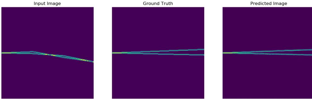
**Figure 3:** An example of correcting for the track multiple scattering using the qSRGAN. The left image is the input to the Generator, the middle image is the true image with no scattering, and the right image is the generated output.
