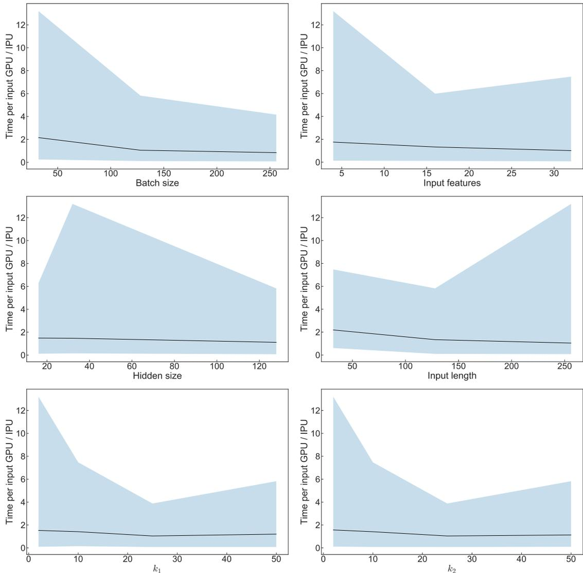
**Figure 8:** Variation of the ratio between the time taken for each input event as a function of batch size, number of input features, hidden layer size, input length, and the size of the two convolutional kernels, for the convolutional neural network. In each case, the black curve indicates the average time ratio when holding the  $x$ -axis value constant, and the coloured band spans the range of possible ratios with constant  $x$ -axis value.
