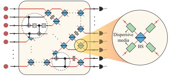
FIG. 1. Schematic of a photonic quantum computing circuit. Linear optics are used for implementing quantum gates and all such optical elements introduce dispersion to the single photon pulses.
