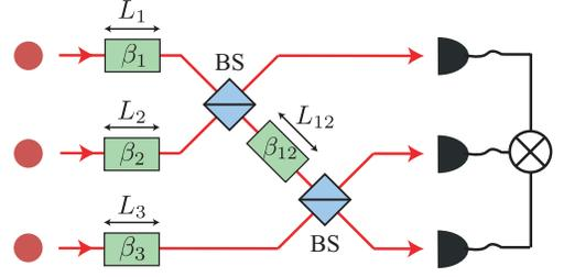
FIG. 5. Schematic of a multi-path quantum interferometer with three single photons and four dispersive media. Under specific sets of conditions, full dispersion cancellation for three-photon quantum interference can be achieved.
