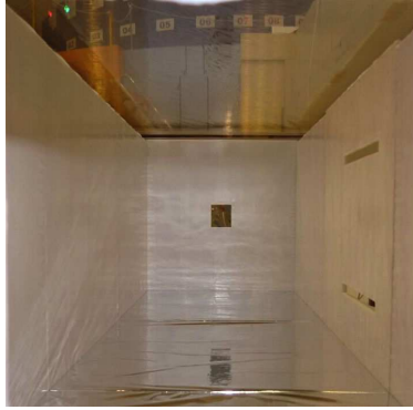
Figure 1. Picture of the inside of the TPC taken from the downstream. The inner wall of the TPC consists of the {}^6\text{LiF} tiles.
