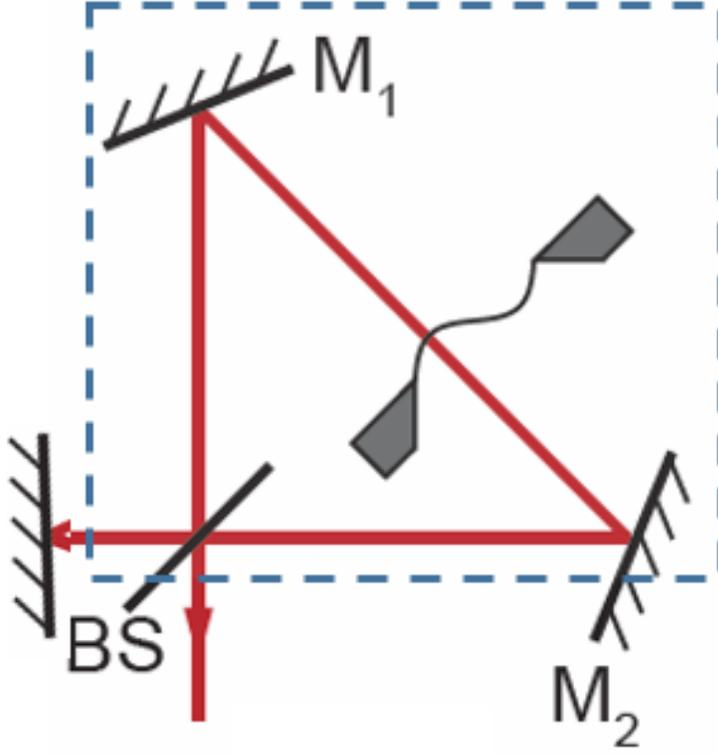
FIG. 1. Schematic of Michelson-Sagnac interferometer. The part marked with a dashed-line rectangle can be considered as an effective input mirror with  $x$ -dependent parameters such that the system can be viewed as a one-sided cavity.
