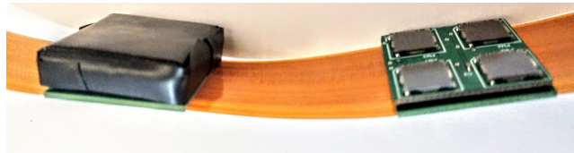
Figure 4. General front-end PCB prototype. The picture shows the SFED card attached to the ribbon card. On the left, the SFED card is wrapped in polyester mylar tape. On the right, the SFED card is unwrapped and the SiPMs distribution is visible
