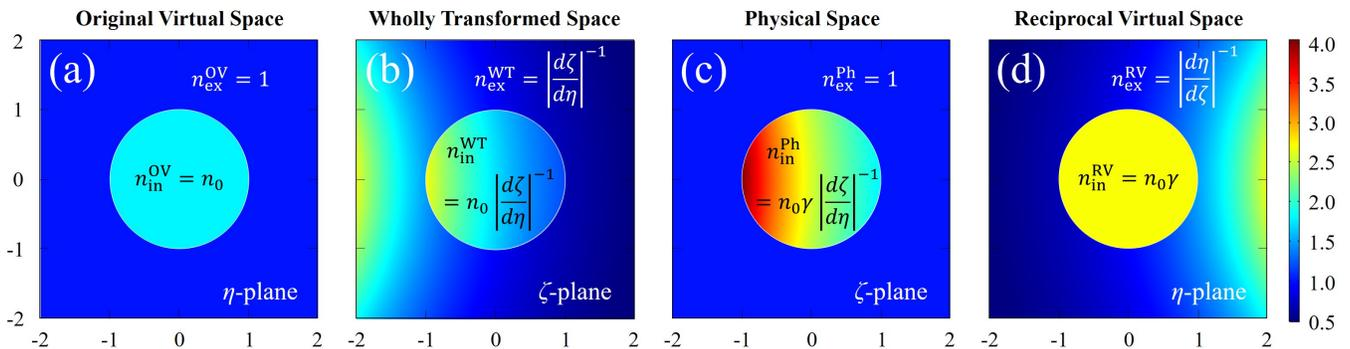
Figure 2. Refractive index profiles in (a) original virtual, (b) wholly transformed, (c) physical, and (d) reciprocal virtual spaces. These pictures were drawn in circle-shaped transformation cavity without a shrinking parameter at  $n_0 = 1.8$ ,  $|\delta| = 0.2$ , and  $\gamma = \gamma_{\min}$ .
