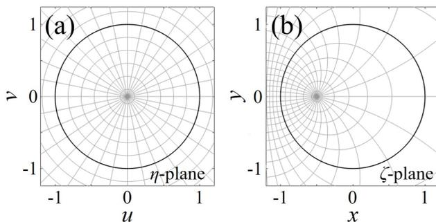
Figure 1. Conceptual diagrams for center-shift conformal transformation from (a)  $\eta$ -plane to (b)  $\zeta$ -plane.
