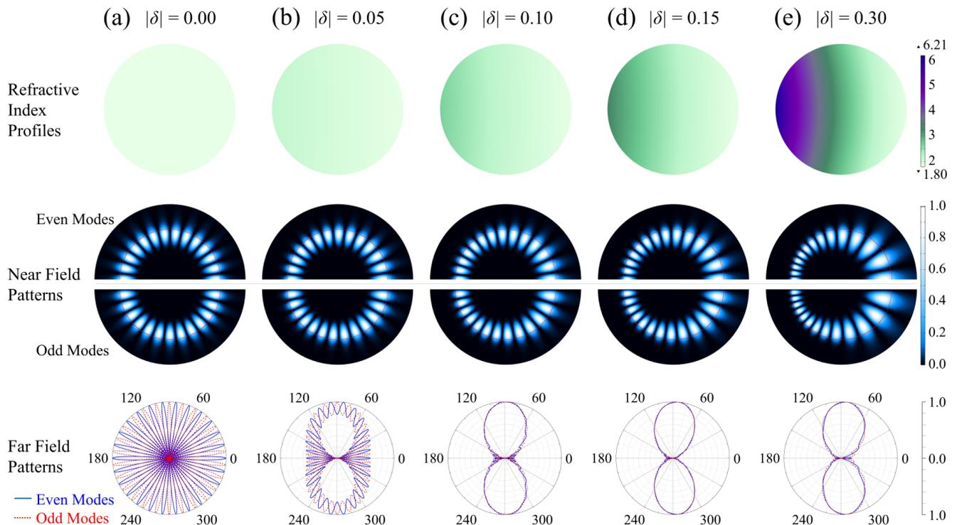
Figure 4. Refractive index profile and near field and far field intensity patterns for the mode pair of  $M(13,1)$  at the shifting parameter (a)  $|\delta| = 0$ , (b) 0.05, (c) 0.10, (d) 0.15, and (e) 0.30 in the  $\gamma$ -type circle-shaped TC with  $n_0 = 1.8$  and  $\gamma = \gamma_{\min}$ . The refractive index of outside cavity set to air. In each step, up-side (down-side) of near field pattern and blue solid (red dashed) line in far-field pattern are the even-parity (odd-parity) mode.
