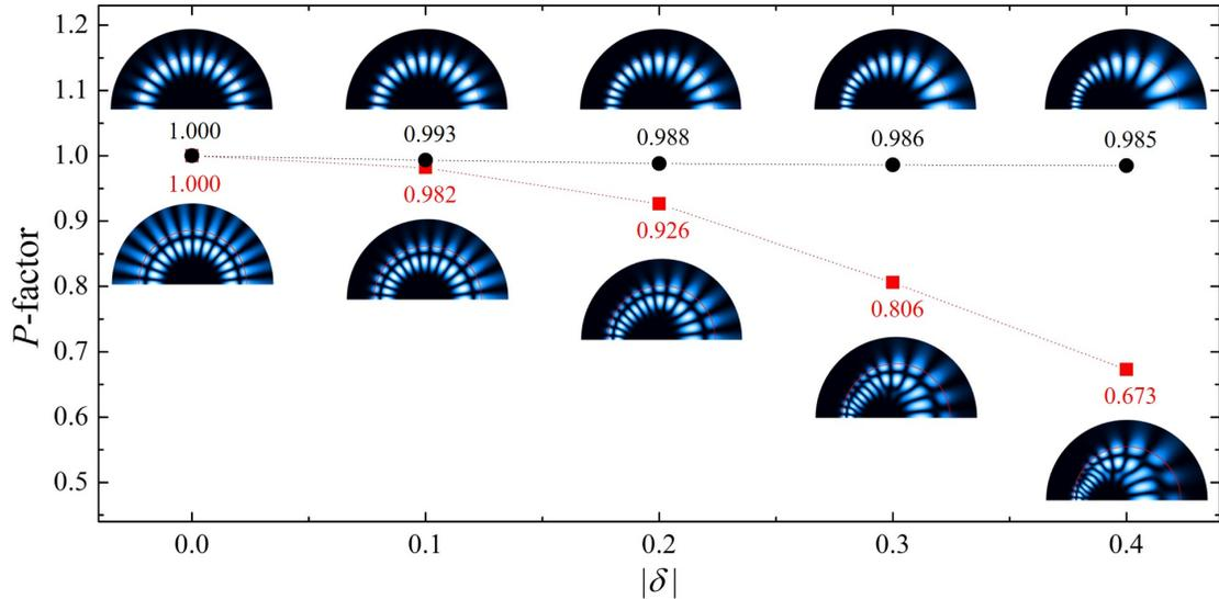
Figure 5. The change of  $P$ -factors for even-parity modes of (a) M(13,1) and (b) M(13,2) according to  $|\delta|$  in  $\gamma$ -type circle-shaped TC with  $n_0 = 1.8$  and  $\gamma = \gamma_{\min}$ . The data pickup domain for  $P$ -factors is set to  $r_{\text{RV}} = 0.8$  and the intensity of the near field patterns is normalized linear scale.
