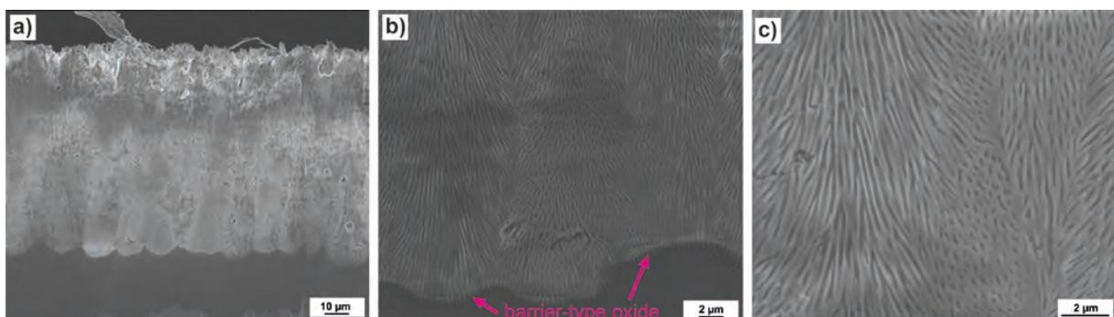
**Figure S6:** SEM images of 1050 P85, porous anodic Al oxide layer formed on AW1050 anodized in 0.1 M  $\text{H}_3\text{PO}_4$  at  $35 \text{ mA cm}^{-2}$  for 6700 s. In this case, the layer presents low degree of ordering with presence of branched pores across the whole layer thickness.
