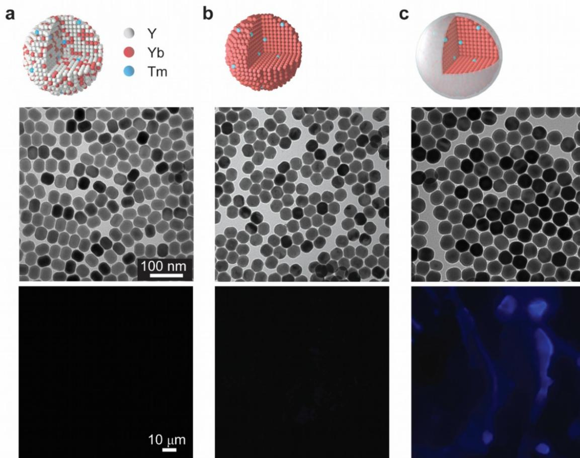
**Figure 1.** TEM and LED-excited UCL images of (a)  $\text{NaY}_{0.79}\text{Yb}_{0.20}\text{Tm}_{0.01}\text{F}_4$ , (b)  $\text{NaYb}_{0.99}\text{Tm}_{0.01}\text{F}_4$  and (c)  $\text{NaYb}_{0.99}\text{Tm}_{0.01}\text{F}_4@\text{NaYF}_4$  UCNPs. Grey, pink and blue dots represent Y, Yb, and Tm ions, respectively. The UCL images were taken by a HUAWEI Mate 10 smartphone in Pro Mode with a blue bandpass filter added before the camera.
