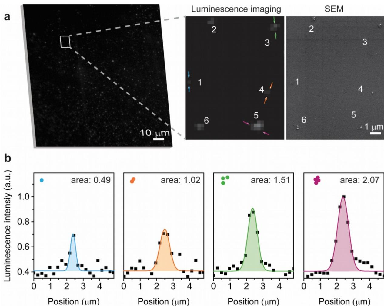
**Figure 4.** Correlative light and electron microscopy images of  $\text{NaYb}_{0.99}\text{Tm}_{0.01}\text{F}_4@\text{NaYF}_4$  UCNPs. (a) UCL and SEM images of the same sample area. (b) The luminescence intensity along the sections of spot 1, 4, 3 and 5 in (a), which has 1-4 UCNPs, respectively. The TGL image was taken under LED excitation with an exposure time of 30 seconds. The intensity has been normalized by the maximum pixel intensity of the 4-UCNP cluster.
