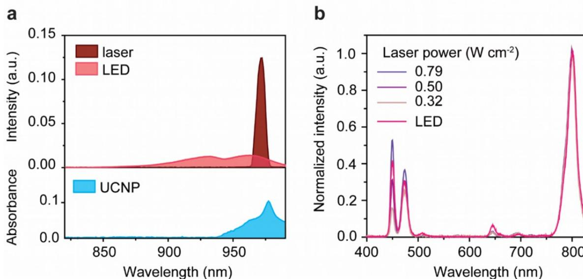
**Figure 2.** Comparison between laser and LED excitation. (a) The excitation spectra of the 976-nm laser and 970-nm LED (top) and the absorption spectrum of  $\text{NaYb}_{0.995}\text{F}_4:\text{Tm}_{0.005}@\text{NaYF}_4$  (bottom). (b) Emission spectra of  $\text{NaYb}_{0.995}\text{F}_4:\text{Tm}_{0.005}@\text{NaYF}_4$  under the laser and LED excitation. Each spectrum was normalized to its emission peak at 800 nm.
