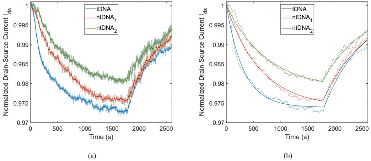
Fig. 11: Specificity analysis of the MC receiver. (a) Real-time sensing response for complementary tDNA, non-complementary ntDNA<sub>1</sub> with single base-pair mismatch, and non-complementary ntDNA<sub>2</sub> with 7 base-pair mismatches (see Table I). At  $t \approx 1800$  s, the DNA solutions are replaced with 0.01xPBS solution to allow dissociation of the hybridised DNAs. (b) Real-time sensing response fitted by the Langmuir adsorption/desorption model, equations (7)-(8).
