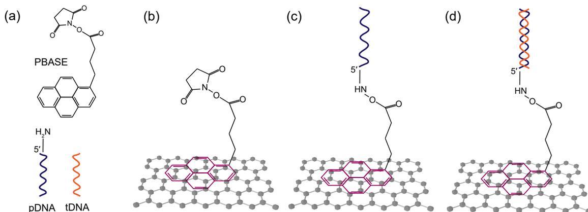
Fig. 8: (a) Molecular structure of PBASE, and conceptual drawing of probe DNA (pDNA) and complementary target DNA (tDNA). (b) Noncovalent binding of PBASE to graphene via  $\pi - \pi$  interaction. (c) Immobilisation of pDNA via conjugation reaction with the succinimide group of PBASE. (d) pDNA-tDNA hybridisation.
