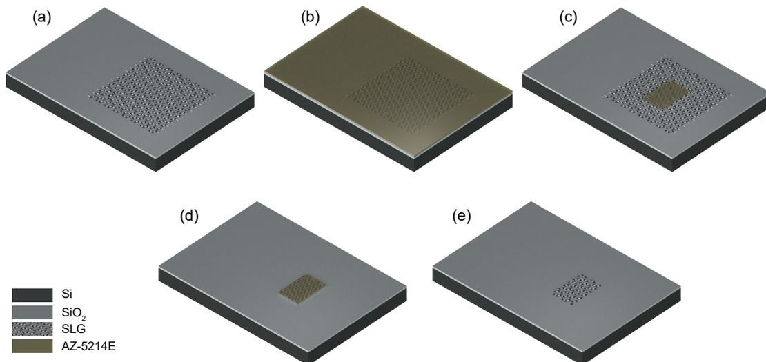
Fig. 1: Process flow for the patterning of SLG channels. (a) SLG transferred on Si/SiO<sub>2</sub> substrate. (b) Coating of sample with photoresist layer. (c) SLG channel pattern defined by optical lithography. (d) SLG channel pattern after RIE etching. (e) Removal of residual photoresist layer from SLG surface, and the resulting SLG channel on the substrate.
