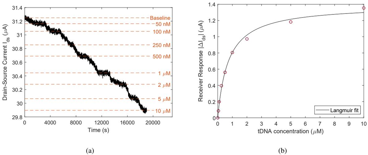
Fig. 10: (a) Real-time sensing response of the MC receiver in terms of drain-source current  $I_{ds}$  with varying concentration of complementary target DNAs (tDNAs). (b) Equilibrium sensing response fitted by the Langmuir adsorption isotherm. Resulting dissociation constant for pDNA-tDNA hybridisation is  $K_D = 730$  nM.
