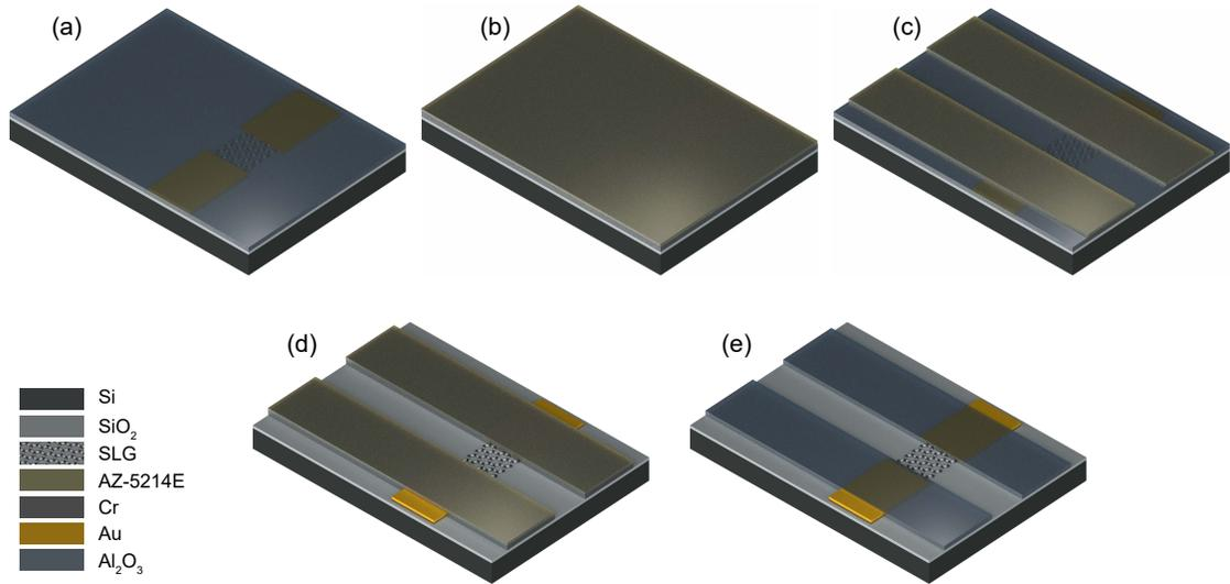
Fig. 3: Process flow for the deposition of insulator. (a) Uniform  $\text{Al}_2\text{O}_3$  film over the sample after ALD. (b) Coating of sample with photoresist layer. (c) Insulator pattern defined by optical lithography. (d) Exposed SLG channel and contacts after wet etching of  $\text{Al}_2\text{O}_3$ . (e) Patterned  $\text{Al}_2\text{O}_3$  film after removal of excess photoresist.
