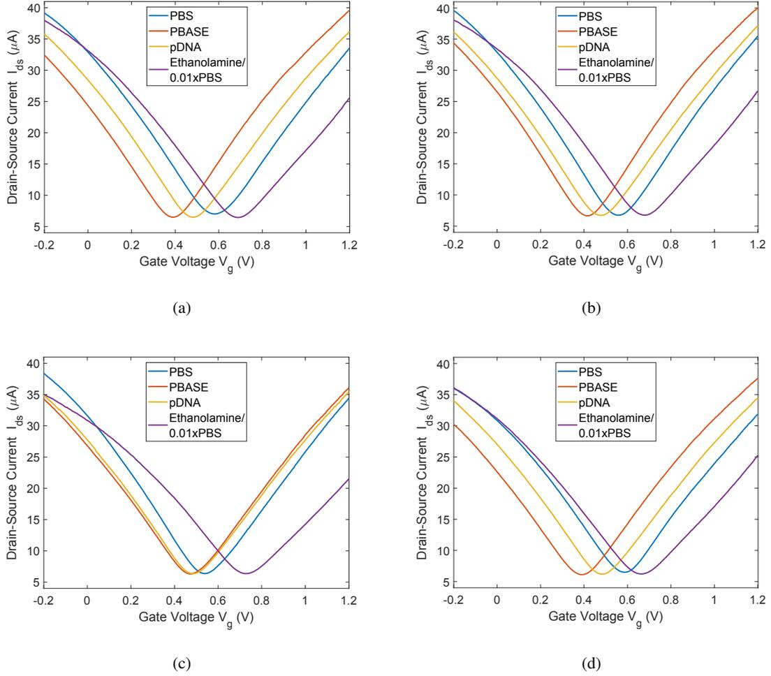
Fig. 9: Transfer characteristics of four channels at different steps of functionalisation in terms of drain-source current  $I_{ds}$  as a function of varying gate voltage  $V_g$  with sweep rate 140 mV/s. In all measurements drain-source voltage is held constant at  $V_{ds} = 0.1$  V.
