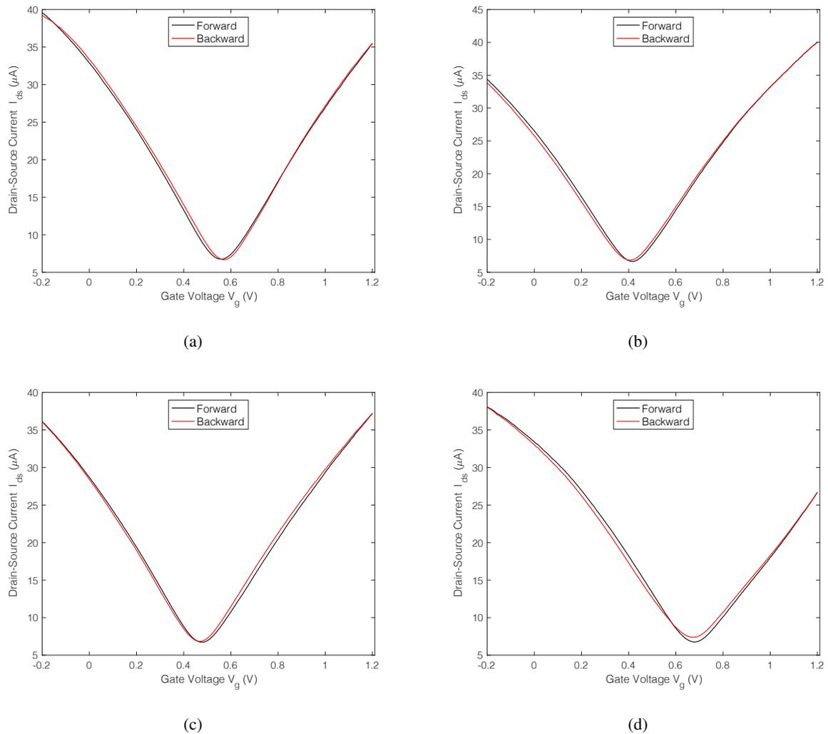
Fig. 15: Hysteresis analysis of the MC receiver: Drain-source current  $I_{ds}$  with forward and backward sweep of gate voltage  $V_g$  at 140 mV/s sweep rate. (a) Before functionalisation. (b) After functionalisation with PBASE. (c) After immobilization of pDNA. (d) After passivation with ethanolamine.
