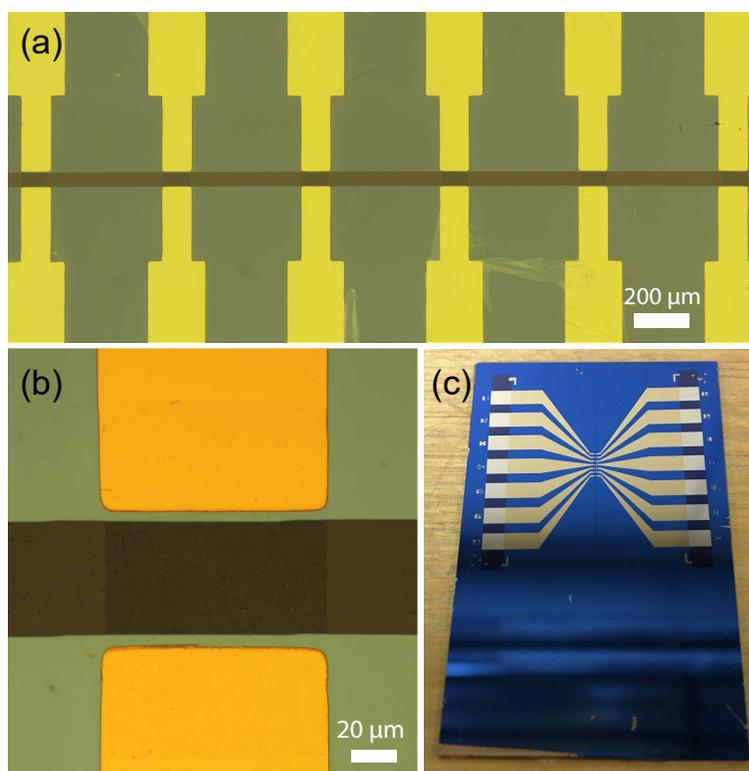
Fig. 4: (a) Optical micrograph of the fabricated GFET channels after  $\text{Al}_2\text{O}_3$  etching process (only six of the seven channels are visible). (b) A closer look into one of the GFET channels. (c) Overall view of the fabricated 7-channel GFET before the bonding of microfluidic PDMS layer.
