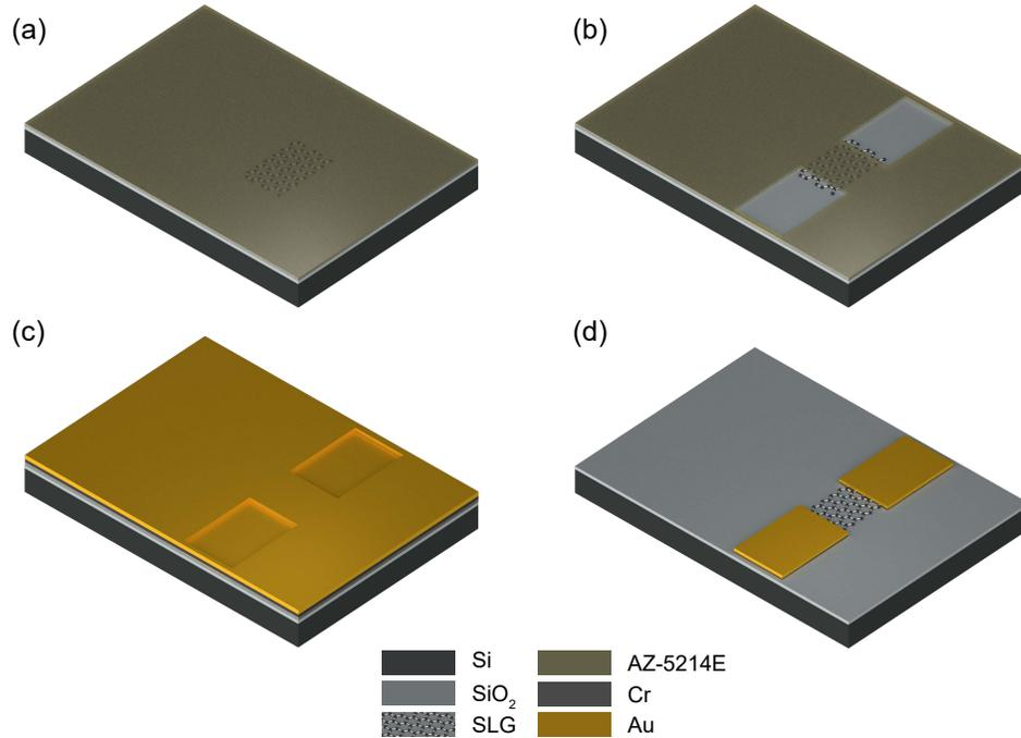
Fig. 2: Process flow for the deposition of contacts. (a) Coating of sample with photoresist layer. (b) Contact pattern defined by optical lithography. (c) Deposition of Cr and Au metal films through thermal evaporation. (d) Patterned contacts after lift-off process.
