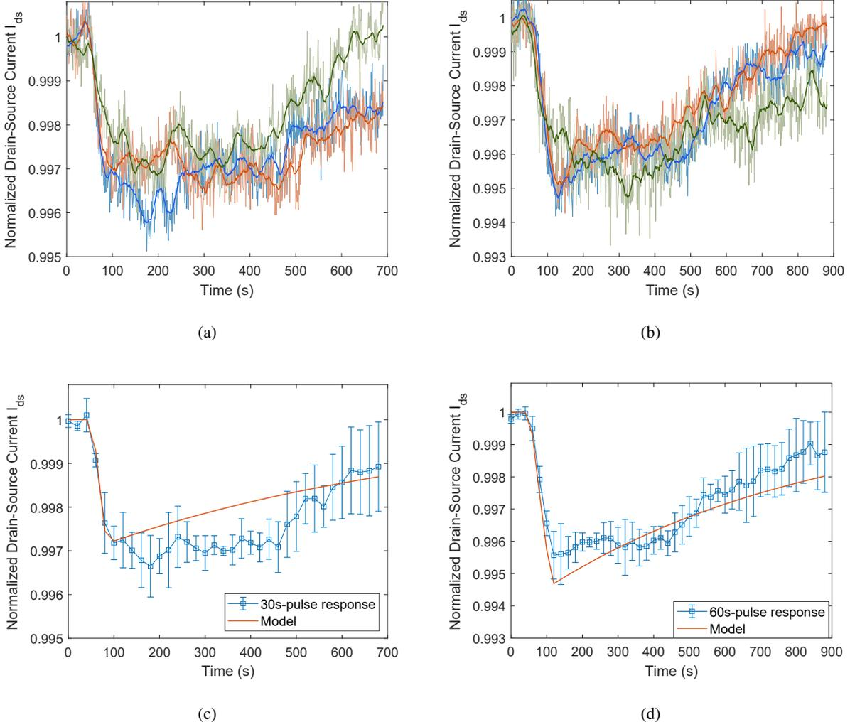
Fig. 12: Normalised pulse response of the MC receiver in terms of drain-source current  $I_{ds}$  with constant operating voltages set to  $V_g = 0$  V and  $V_{ds} = 0.1$  V. (a, b) Three independent measurements taken from the same channel for 30-second-long and 60-second-long  $1 \mu\text{M}$  tDNA pulses, respectively. (c, d) Pulse responses fitted by the normalised output of the transformed model given in (13).
