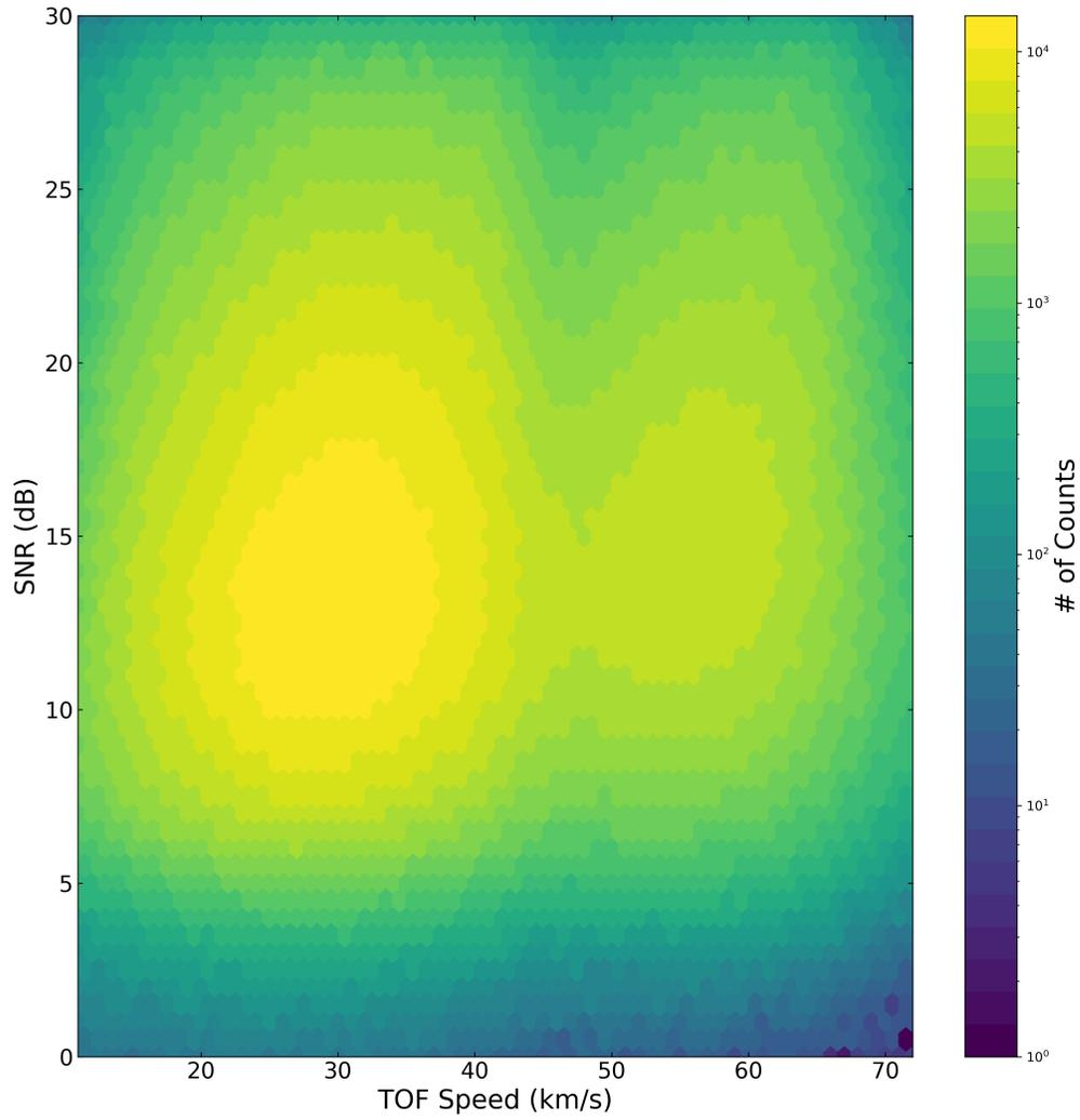
**Figure 15.** The overall log distribution of signal-to-noise ratio of 12 million CMOR echoes where TOF speeds were measurable from data collected between 2010-2019. The broadening in the distribution at higher speeds shows that the proportion of high-speed echoes in the data set increases with increasing SNR.
