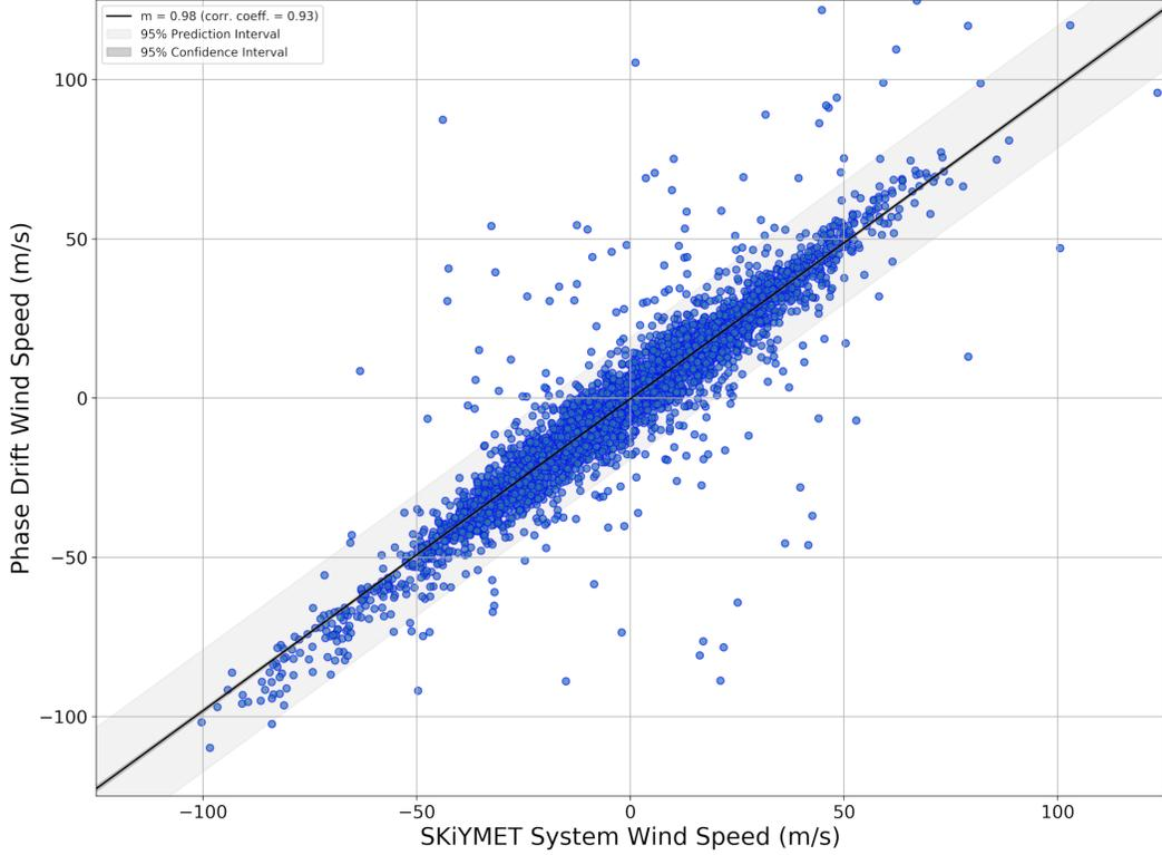
**Figure 4.** Radial, line-of-sight wind speeds calculated by the phase-drift method described in this paper are compared to wind speeds for the same 4775 echos automatically calculated by the SKiYMET system following the technique described in Hocking et al. (2001). These are from CMOR echos collected on October 8, 2012.
