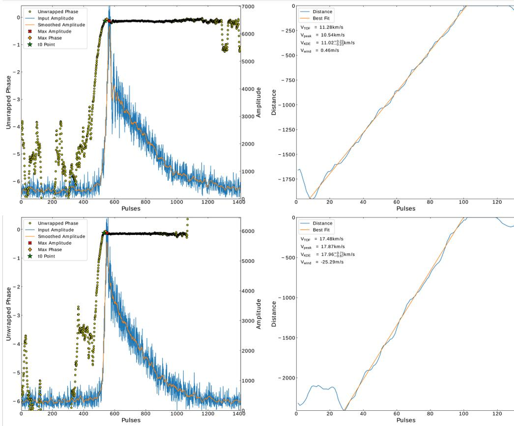
**Figure 13.** PSSST speed results for echo examples having TOF speeds of  $11.28 \pm N/A$  km/s (top panels) and  $17.48 \pm 1.12$  km/s (bottom panels). The radial neutral wind drift is also shown ( $V_{wind}$ ).
