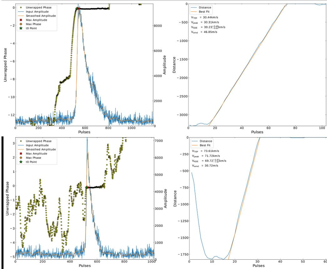
**Figure 14.** PSSST results for echoes with TOF speeds of  $30.44 \pm 0.44$  km/s (top panels) and  $73.61 \pm 471.4$  km/s (bottom panels). The large error associated with the TOF solution for the bottom echo is a sign that the TOF algorithm has failed due to poor specular point geometry where all points are near the same point on the trail.
