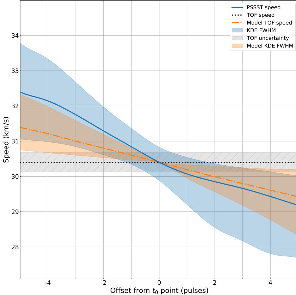
**Figure 5.** The PSSST echo speed sensitivity to offset from the automated  $t_0$  pick location for a real echo with a TOF speed of  $30.44 \pm 0.28$  km/s (solid line). The true  $t_0$  location is located at the KDE FWHM minimum and is consistent with the auto-pick. Also shown are the results for a noise-free synthetic echo with the same speed (dash-dot line). Here we define a negative offset as earlier than the auto-pick  $t_0$  point and a positive offset as later.
