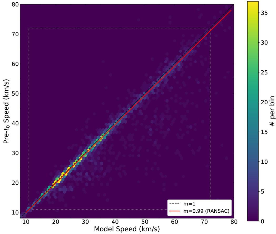
**Figure 9.** A density plot of pre- $t_0$  speeds determined from the PSSST method versus model echo speeds for synthetic data conditioned to match height vs. speed of real echoes detected on Oct 9, 2012. The dotted square shows the 11 km/s and 72 km/s extreme velocity bins where objects are in geocentric orbits (lower) or hyperbolic relative to the sun (upper).
