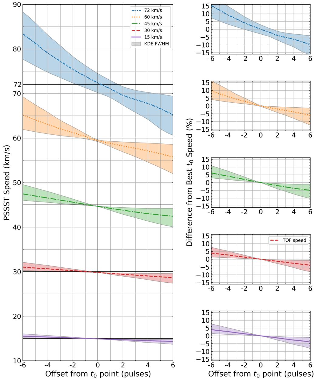
**Figure 6.** Sensitivity of the  $t_0$  point pick on PSSST speeds shown for synthetic and noise-free echoes at true speeds of 15, 30, 45, 60, and 72 km/s, respectively. The left panel shows the PSSST results at different  $t_0$  offsets, while the right panels show the percentage differences as the  $t_0$  point is varied. Here we define a negative offset as earlier than the auto-pick  $t_0$  point and a positive offset as later.
