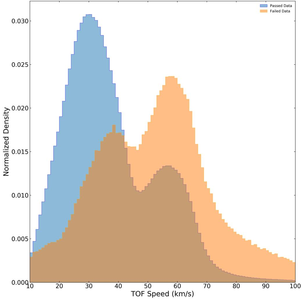
**Figure 16.** The relative fraction of echoes per one km/s bin as a function of TOF speed showing where the PSSST algorithm produced a speed estimate (passed) and failed to converge to a speed estimate (failed).
