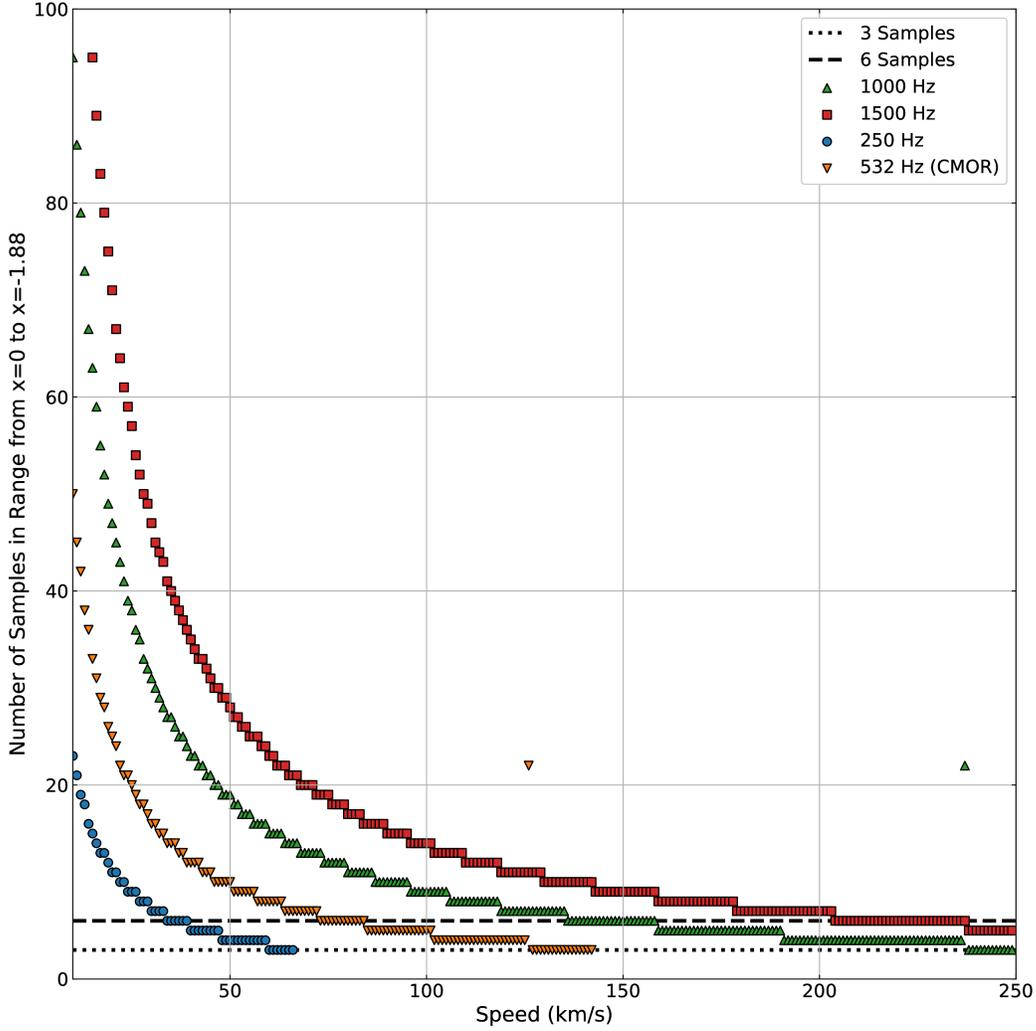
**Figure 2.** The number of pulses (samples) in the first  $2\pi$  phase increment after the  $t_0$  ( $x = 0 \rightarrow x = -1.88$ ) versus meteoroid speed. Here the range is 100 km and the radar wavelength is 10 m in all cases. Although a minimum of three samples are typically required, aliasing can occur when the number of samples changes from four to three. Three (absolute) and six (practical) sample aliasing limits are shown by the dotted and dashed lines respectively.
