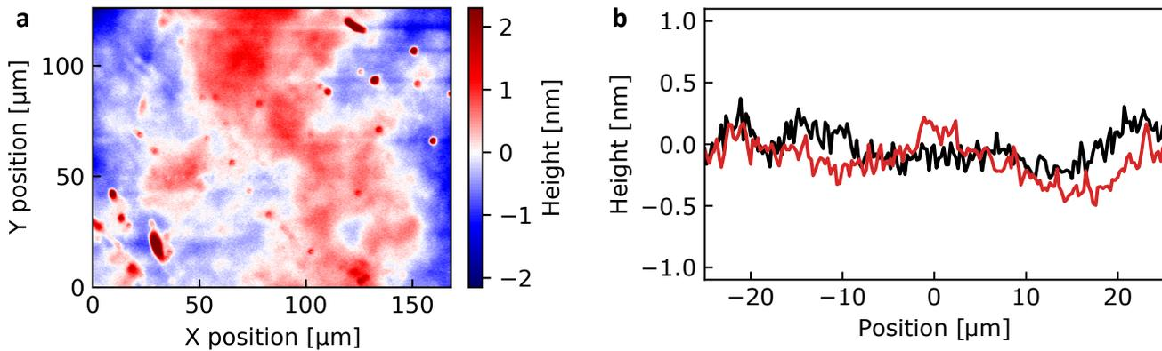
FIG. 7. **Crystal properties.** **a.** Surface height profile of the YSO membrane after transfer to the mirror. At its center, the membrane is fully bonded to the mirror and shows excellent flatness. Apart from a few dust particles that might be removed by further cleaning (red dots), the surface height variation is well below 1 nm. **b.** As can be seen from line cuts at the center, the surface roughness is below 0.2 nm over the  $\simeq 10 \mu\text{m}$  mode diameter of our resonator.
