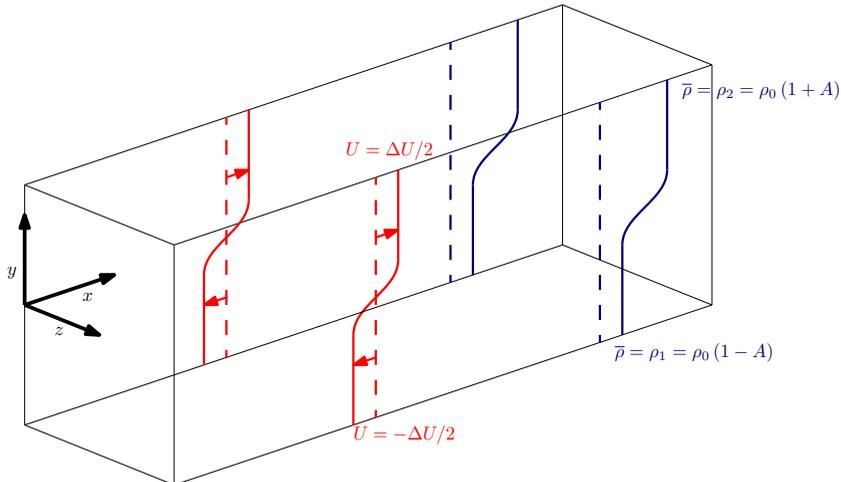
FIGURE 1. Variable-density mixing layer simulation set-up and coordinate system.
