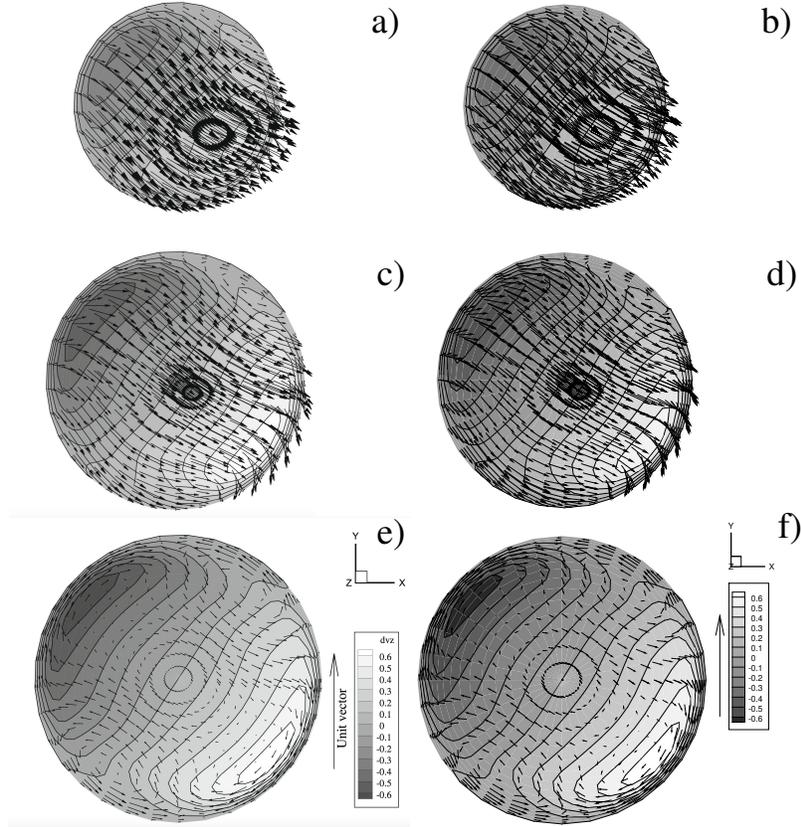
Figure 9: Flow in a precessing, spinning sphere at  $\Gamma = 0.1$  and  $Re = 500$ . The velocity vectors of the field rotating with the spinning sphere  $\mathbf{v}$  are reported in the sections  $z = -0.66$ , a) and d);  $z = -0.33$ , b) and e);  $z = 0$ , c) and f). The contours are for the velocity component  $v_z$ . a), c) and e) are the results adapted from Fig. 7 of [42], b) ,d) and f), present results.
