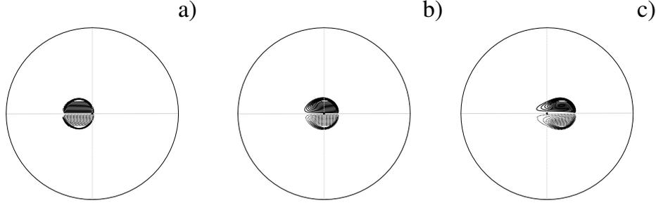
Figure 4: Time evolution of the Hill vortex at  $Re = 2500$  in the longitudinal sections  $\theta = 0, \pi$ ; longitudinal vorticity ( $\Delta\omega_\theta = \pm 0.4$ ) ..... for negative values; a) )  $t = 0.5$ , b)  $t = 1.$ , c)  $t = 1.5$ . Initial centre of the vortex:  $\theta_C = \pi$ ,  $r_C = 1$ ,  $\phi_C = \pi/2$ . Hereinafter, the black bullet indicates the origin of the spherical system.
