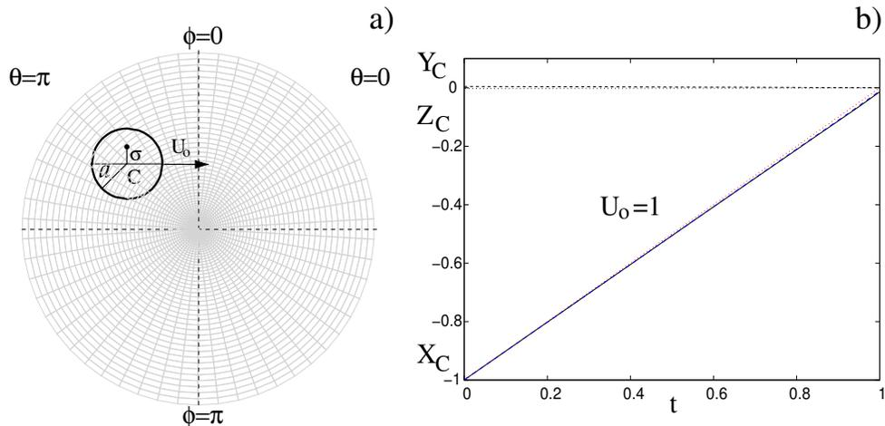
Figure 3: a) Sketch of the Hill vortex setup in the longitudinal sections  $\theta = 0, \pi$  of the spherical domain. b) Time evolution of the vortex centre coordinates for the case at  $Re = 2500$  with  $\theta_C = \pi$ ,  $r_C = 1$ ,  $\phi_C = \pi/2$ . —  $X_C = r_C \cos \theta_C \sin \phi_C$ , ----  $X_C$  from the code in Cartesian coordinates [41], thin ..... theoretical  $X_C$ ; ----  $Y_C = r_C \sin \theta_C \sin \phi_C$ ; -.-  $Z_C = r_C \cos \phi_C$ .
