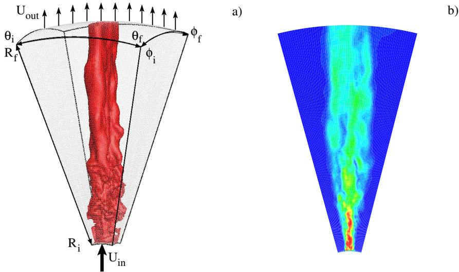
Figure 12: a) Computational set-up for the space developing jet. The isosurface is velocity magnitude  $|\mathbf{u}| = 0.2$ . b) Instantaneous snapshot plane section ( $\theta = (\Theta_i + \Theta_f)/2$ ) of velocity magnitude (from blue to red)  $\Delta |\mathbf{u}| = 0.1$ .
