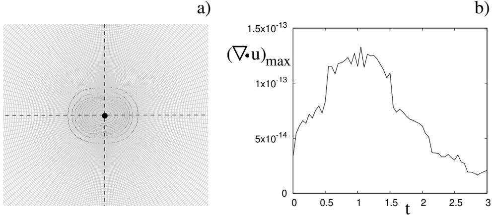
Figure 8: a) Zoom of velocity magnitude ( $\Delta u = 0.1$ ) of a Hill vortex at  $Re = 2500$  and  $t = 1$  in the longitudinal sections  $\theta = 0, \pi$ ; the computational mesh is refined on purpose around the singular points. b) Time evolution of the maximum divergence of the velocity field. Initial centre of the vortex:  $\theta_C = \pi$ ,  $r_C = 1$ ,  $\phi_C = \pi/2$ .
