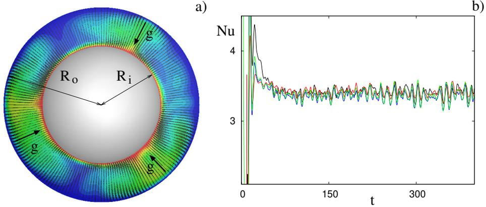
Figure 11: a) Section through the meridional planes  $\theta = 0, \pi$  of temperature contours ( $\Delta T = 0.1$ ) overlaid with velocity vectors for the flow at  $\eta = R_i/R_o = 0.6$ ,  $Ra = 3 \times 10^4$  and  $Pr = 1..$  Grid  $129 \times 97 \times 97$ . b) Time evolution of the Nusselt numbers: — value computed at the inner surface, — value computed at the outer surface, — value computed from  $\epsilon_u$ , — value computed from  $\epsilon_T$ .
