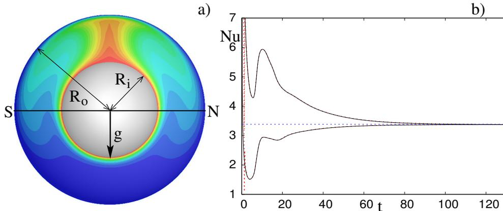
Figure 10: a) Section through the meridional planes  $\theta = 0, \pi$  of temperature contours ( $\Delta T = 0.1$ ) for the flow at  $\eta = R_i/R_o = 0.5$ ,  $Ra = 10^5$  and  $Pr = 0.7$ . Grid  $65 \times 49 \times 49$ . b) Time evolution of the Nusselt numbers ——— simulation with the gravity aligned with the polar axis, - - - gravity perpendicular to the polar axis, ····· reference value of  $Nu = 3.4012$  from [43].
