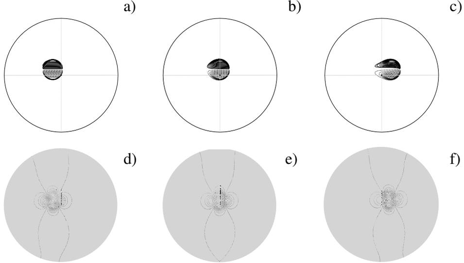
Figure 7: Time evolution of the Hill vortex at  $Re = 2500$  in the longitudinal sections  $\theta = 0, \pi$ ; top panels show longitudinal vorticity ( $\Delta\omega_\theta = \pm 0.4$ ) ..... for negative values; ( $\Delta u = 0.1$ ) bottom panels for pressure ( $\Delta p = 0.02$ ); the background mesh is shown with light gray lines. a) and d)  $t = 0.5$ , b) and e)  $t = 1.$ , c) and f)  $t = 1.5$ . Initial centre of the vortex:  $\theta_C = \pi$ ,  $r_C = 1$ ,  $\phi_C = 2\pi/3$ .
