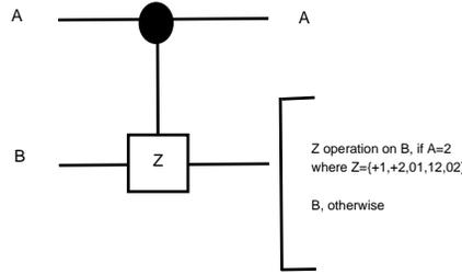
**Figure 4:** Circuit Representation of 2-qutrit M-S gate
