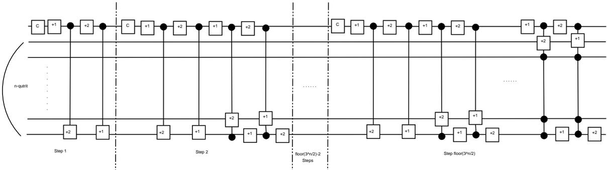
**Figure 12:** Generalization of Quantum circuit for  $\lfloor 3^n/2 \rfloor$  steps of the LQW on a  $n$  qutrit ternary system with a fixed initial state  $|\uparrow\rangle \otimes |x = 0\rangle \equiv |\uparrow\rangle \otimes |(n - 1) \text{ times } 0's)$ .
