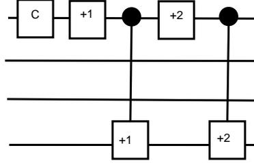
**Figure 6:** Quantum circuit for the first step of LQW on four qutrits as given in Table. 3
