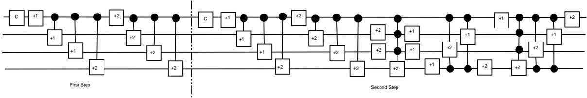
**Figure 11:** Quantum circuit for first two steps of the LQW on a four qutrit ternary system with a fixed initial state  $|\uparrow\rangle \otimes |x = 0\rangle \equiv |\uparrow\rangle \otimes |000\rangle$ . The position state mapping is shown in Table. 8
