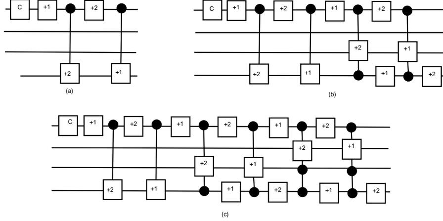
**Figure 10:** (a)Quantum circuit for the first steps of LQW on four qutrits as shown in Table. 6; (b)Quantum circuit for the second-fourth steps of LQW on four qutrits as shown in Table. 6 (c)Quantum circuit for the fifth-thirteenth steps of LQW on four qutrits as shown in Table. 6
