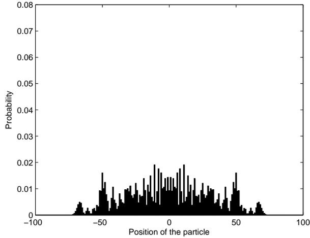
**Figure 2:** Lazy quantum walks on a line using three-state DFT coin in ternary system, after 100 steps
