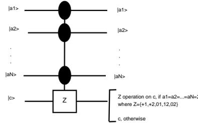
**Figure 5:** Circuit Representation of multi-controlled M-S gate
