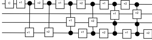
**Figure 8:** Quantum circuit for the fifth-thirteenth steps of LQW on four qutrits as shown in Table. 5
