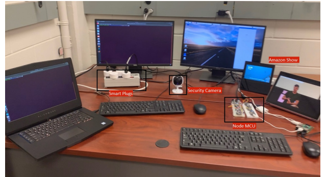
Fig. 7. IoT testbed consisting of NodeMCUs, smart switches, security camera, Amazon Echo Show, laptop, tablet, and Raspberry Pi.
