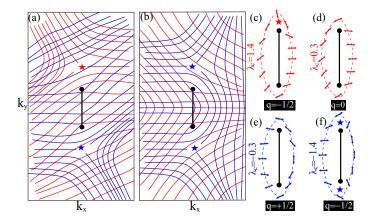
FIG. 3. (a) and (b) Polarization fields extrated from the model respectively in Eq. (3) and Eq. (4), with  $\gamma=1$  and  $\kappa=0.8$ . Two iso-eigenvalue contours are selected in (a) and (b), on which the polarizations fields are shown in (c)-(f), with q=-1/2,0,0,-1/2, respectively.
