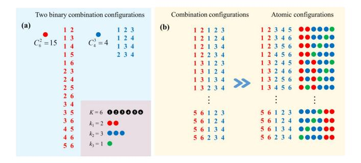
**FIG. 2**. (Color online) The enumeration of ternary site-occupancy configurations for K = 6,  $k_1 = 2$  (red),  $k_2 = 3$  (blue),  $k_3 = 1$  (green). (a) The binary combination configurations for red and blue color. (b) The conversion of combination configurations to atomic configurations.
