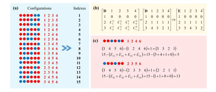
**FIG. 3**. (Color online) The conversion of binary site-occupancy configurations to consecutive integers (indexes) for K = 6,  $k_1 = 4$  (red),  $k_2 = 2$  (blue). (a) The atomic configurations and its corresponding indexes. (b) The constructing flow of matrix **E**. (c) Two specific examples of atomic configurations to integers.
