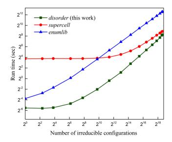
**FIG. 6.** (Color online) The run time of *disorder*, *supercell* and *enumlib* codes as a function of the number of irreducible configurations in a  $2\times2\times2$  FCC lattice. One can see that the *disorder* code (this work) has the lowest run time in the whole range of the number of irreducible configurations.
