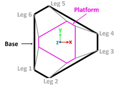
Figure 5. Hexapod with platform in  $[0\text{mm } 0\text{mm } 0\text{mm } 0^\circ 0^\circ 0^\circ]$  pose (top view)
