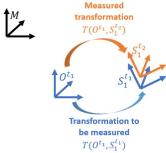
**Figure 1.** Illustration of the conventional pose measurement method to measure the coordinate frame of an arbitrary pose  $S_1$  with respect to a coordinate frame  $O$
