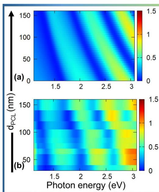
**Figure 4.** Calculated and measured reflectance of ML2 thin-film.
