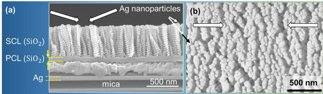
**Figure 2.** SEM micrograph of the ML2 thin-film. (a) cross-sectional; and (b) top view
