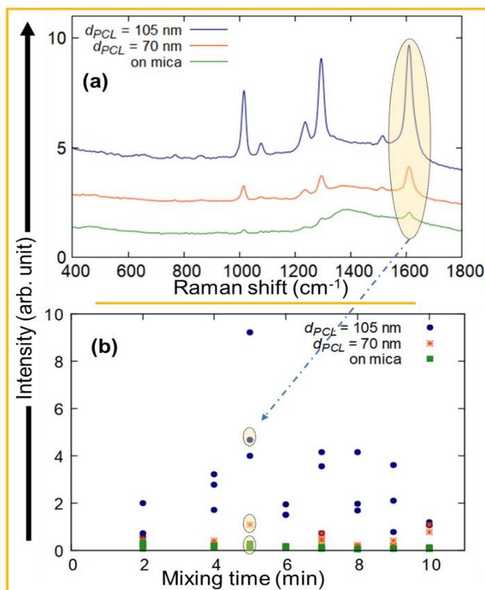
**Figure 7.** (a) SERS spectra of ML2 thin-film ( $d_{PCL} = 70$  nm, and 105 nm) and AgNRAs dispersion gel after stirring for 5 min; (b) SERS peak intensity ( $1624\text{ cm}^{-1}$ ) vs. stirring time ML2 thin-film ( $d_{PCL} = 70$  nm, and 105 nm) and AgNRAs dispersion gel. The data was recorded after 60 min of dropping BPY solution.
