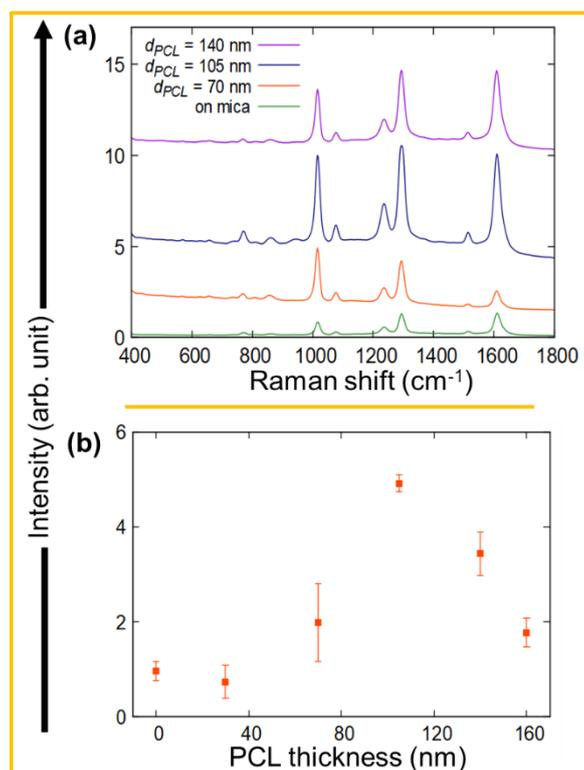
**Figure 5.** (a) SERS spectra of BPY on ML2 thin-film with  $d_{PCL} = 70$  nm, 105 nm, 140 nm, and AgNRAs on a mica substrate in gel of thickness 0.5 mm. The data was recorded after 60 min of dropping BPY solution; (b) SERS peak intensity ( $1624\text{ cm}^{-1}$ ) vs PCL film thickness.
