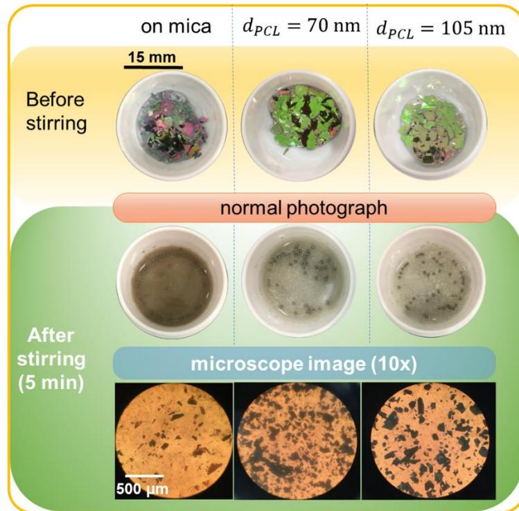
**Figure 6.** Normal photograph and microscopic image of the ML2 thin-film dispersion gel, with different  $d_{PCL}$  thicknesses, before and after stirring.
