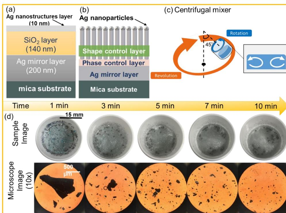
**Figure 1.** A schematic diagram of the cross section of (a) ML1; and (b) ML2 thin-films; (c) a schematic diagram of the centrifugal mixing. Arrows represent the state of the vertical and vertical flow generated in the sample; (d) actual photograph and microscopic image of the ML1 flake dispersion gel for different stirring time.
