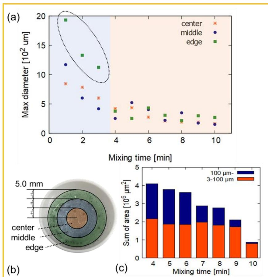
**Figure 3.** (a) Variation in maximum diameter of the dispersed flakes with stirring time; (b) schematic diagram of the division of regions for the particle size measurement; (c) dependence of the total area of thin-film flakes on stirring time. The total height of the bar represents the total area of each sample. The orange part represents the area of thin-film flakes with a particle size of 3-100  $\mu\text{m}$  and the blue part with more than 100  $\mu\text{m}$ .
